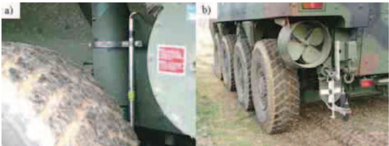
Fig. 3. Location of sensors outside vehicle: a) linear displacement inductive sensor; b) the vehicle speed optical sensor
