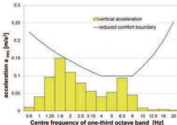
Fig. 9. The acceleration RMS value spectrum chart for driver seat – simulation, parameters:  $G_w=0.000006 \text{ m}^3$ ,  $w=2.18$
