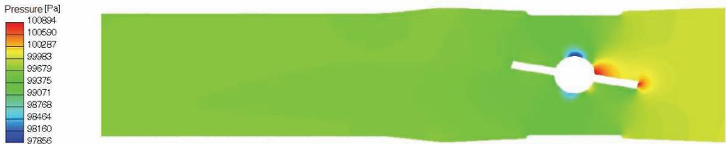
Fig. 8. Pressure distribution in the throttle cross-section for the angle of  $80^\circ$
