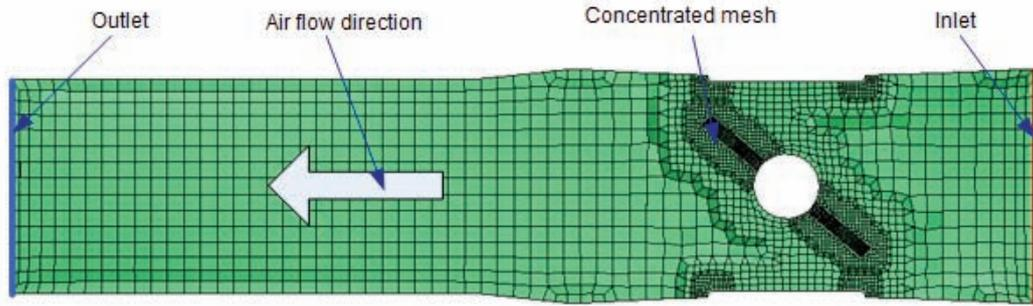
Fig. 3. Mesh cross-sectional view with the boundary conditions marked
