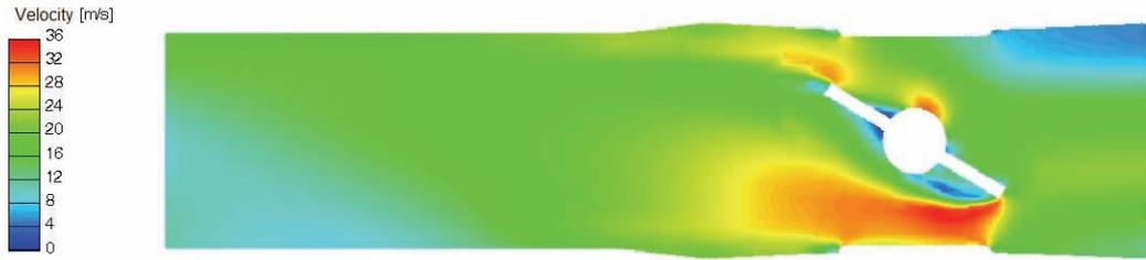
Fig. 12. Velocity distribution in the throttle cross-section for the angle of  $60^\circ$
