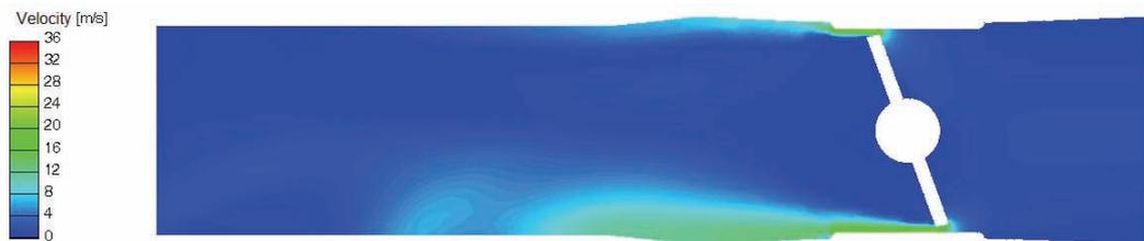
Fig. 10. Velocity distribution in the throttle cross-section for the angle of  $20^\circ$
