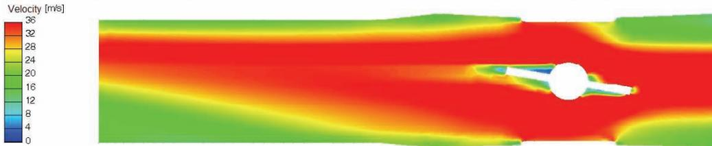
Fig. 13. Velocity distribution in the throttle cross-section for the angle of  $80^\circ$
