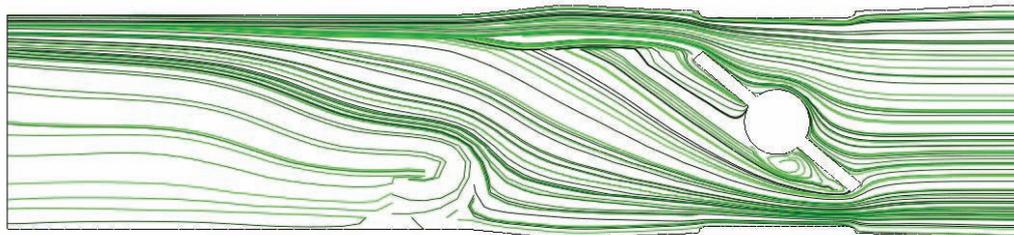
Fig. 15. Stream line distribution in the throttle cross-section for the angle  $50^\circ$
