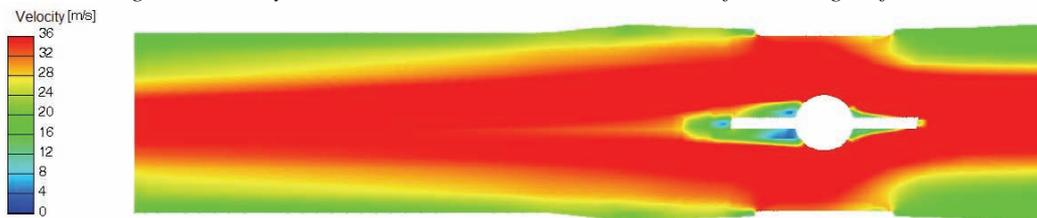
Fig. 14. Velocity distribution in the throttle cross-section for the angle of  $90^\circ$
