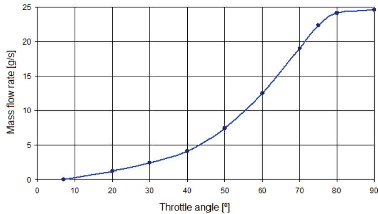
Fig. 17. Dependence of the mass flow rate on the angle of the throttle position
