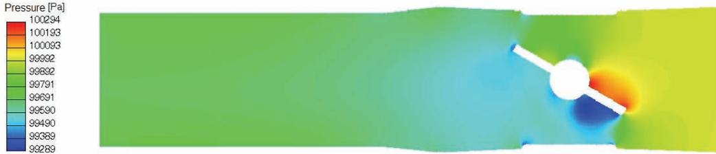
Fig. 7. Pressure distribution in the throttle cross-section for the angle of  $60^\circ$
