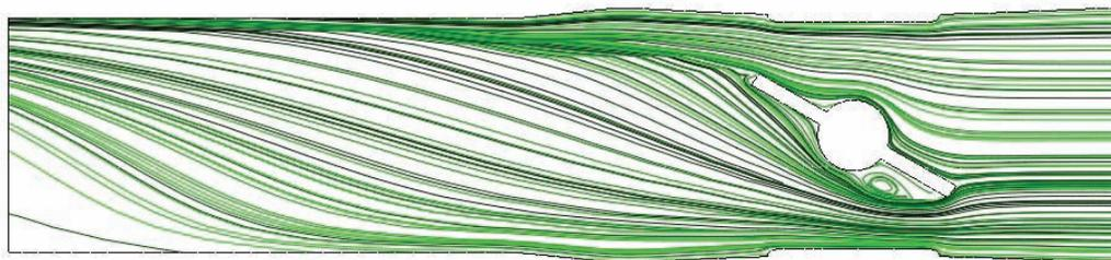
Fig. 16. Stream line distribution in the throttle cross-section for the angle  $60^\circ$
