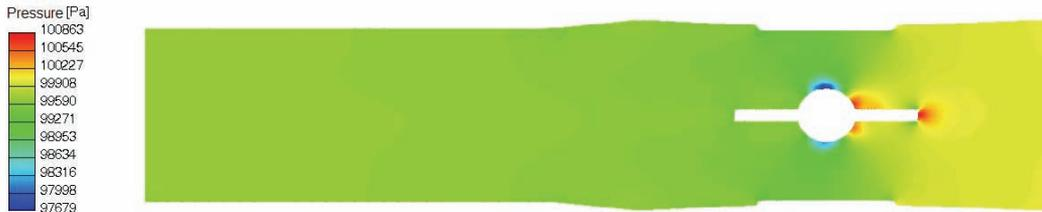
Fig. 9. Pressure distribution in the throttle cross-section for the angle of  $90^\circ$
