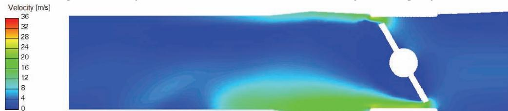
Fig. 11. Velocity distribution in the throttle cross-section for the angle of  $40^\circ$
