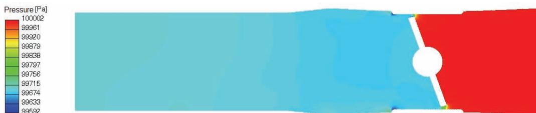
Fig. 5. Pressure distribution in the throttle cross- section for the angle of 20°
