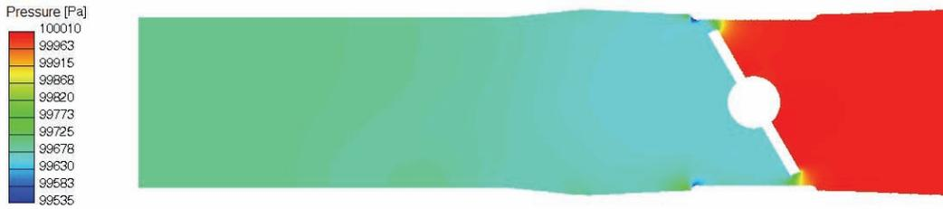
Fig. 6. Pressure distribution in the throttle cross-section for the angle of  $40^\circ$
