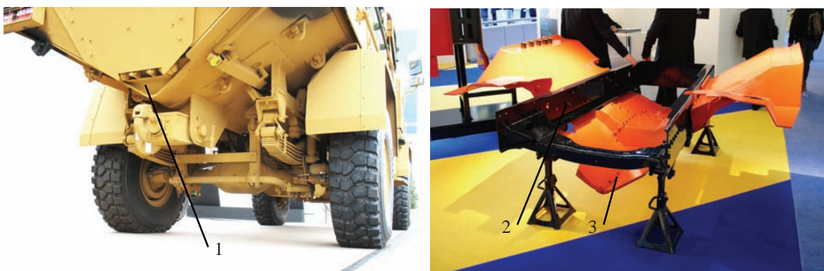
Fig. 4. Hull underside (on the left) and a V-shaped armour: 1 – hull; 2 – frame; 3 – armour (shield)
