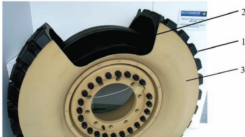
Fig. 6. MRAP (mine resistant ambush protected) reinforced wheel: 1 – tyre, 2 – insert dissipating explosion energy, 3 – tyre shield
