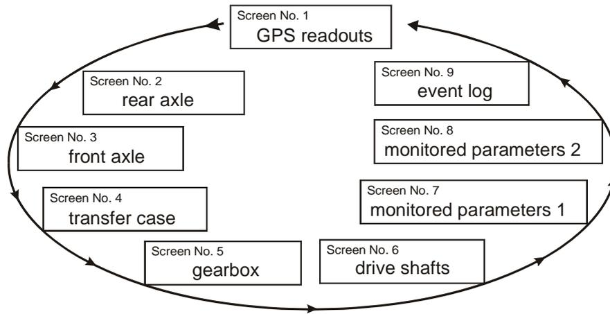
Fig. 4. Hierarchical structure of ALS screens
