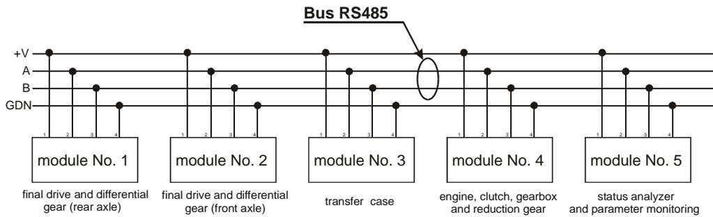
Fig. 1. Functional structure of the diagnostic system and the data transmission system with an indication of the main system components, +V – power supply, GDN – ground, A, B – bus signal line
