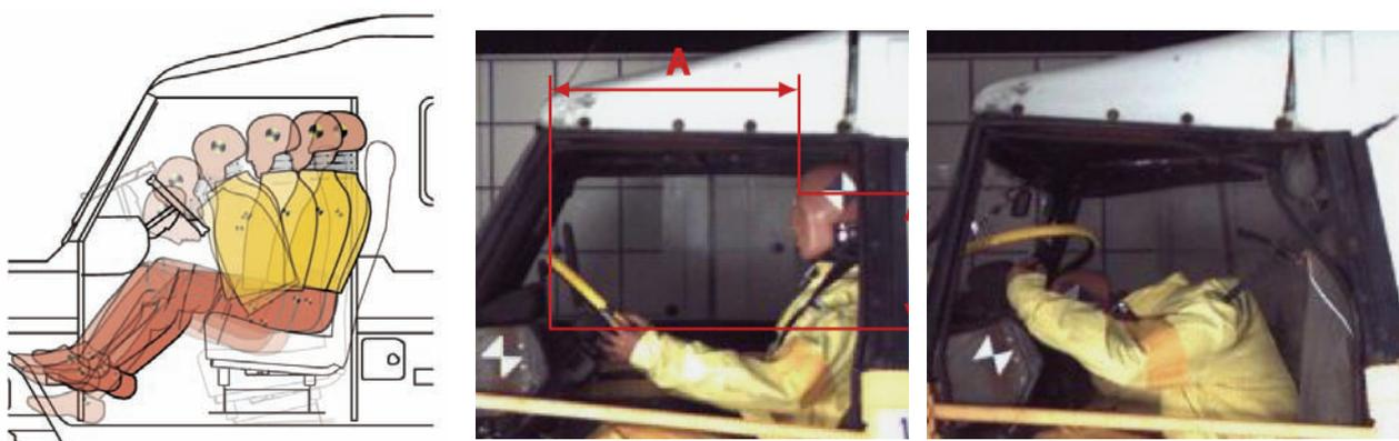
Fig.4.1. Outline of the driver's cab in the Honker and the following stages of the dummy displacement during the experiment; distance between the initial head position and the impact point:  $A=0,53$  m,  $B=0,25$  m
