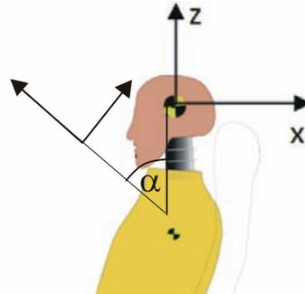
Fig. 4.7. Change of the head sensor axis position
