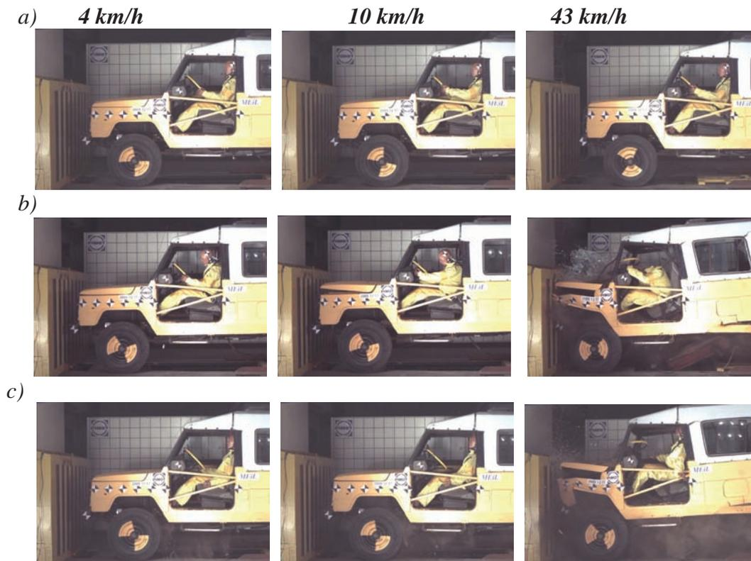
Fig. 3.1. Photos illustrating the dummy displacement and vehicle body deformation in frontal impact barrier test: a – condition before the collision, b – maximum dummy shift forward, c – maximum dummy shift backwards
