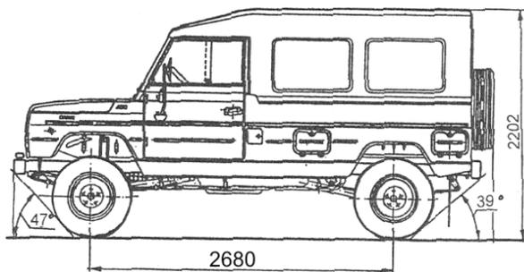
Fig.2.1. Test object and its basic dimensions [1]
