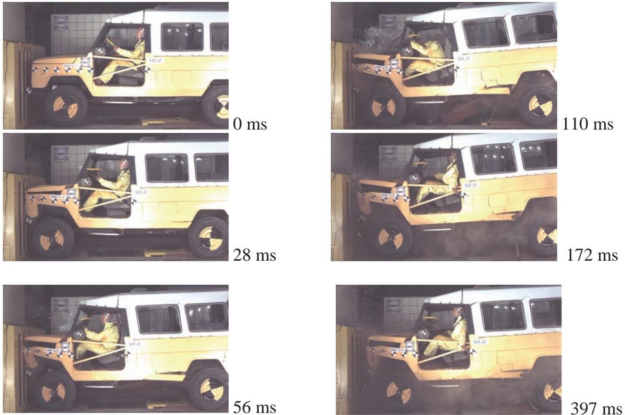
Fig. 3.2 Characteristic stages of the dummy and the vehicle motion in barrier impact at the speed of 43 km/h (numbers next to the video frames indicate current time as in table 3.1).
