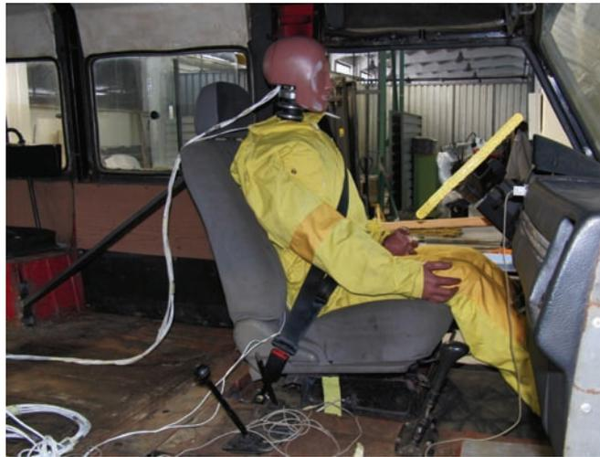
*Fig. 2.4. Arrangement of a dummy with sensors during preparation for the tests*
