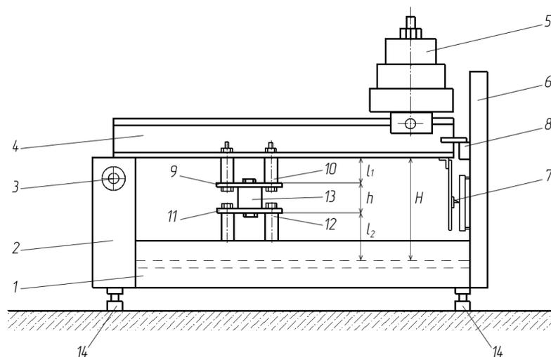
Fig. 1. Vibration isolators' test bench scheme
