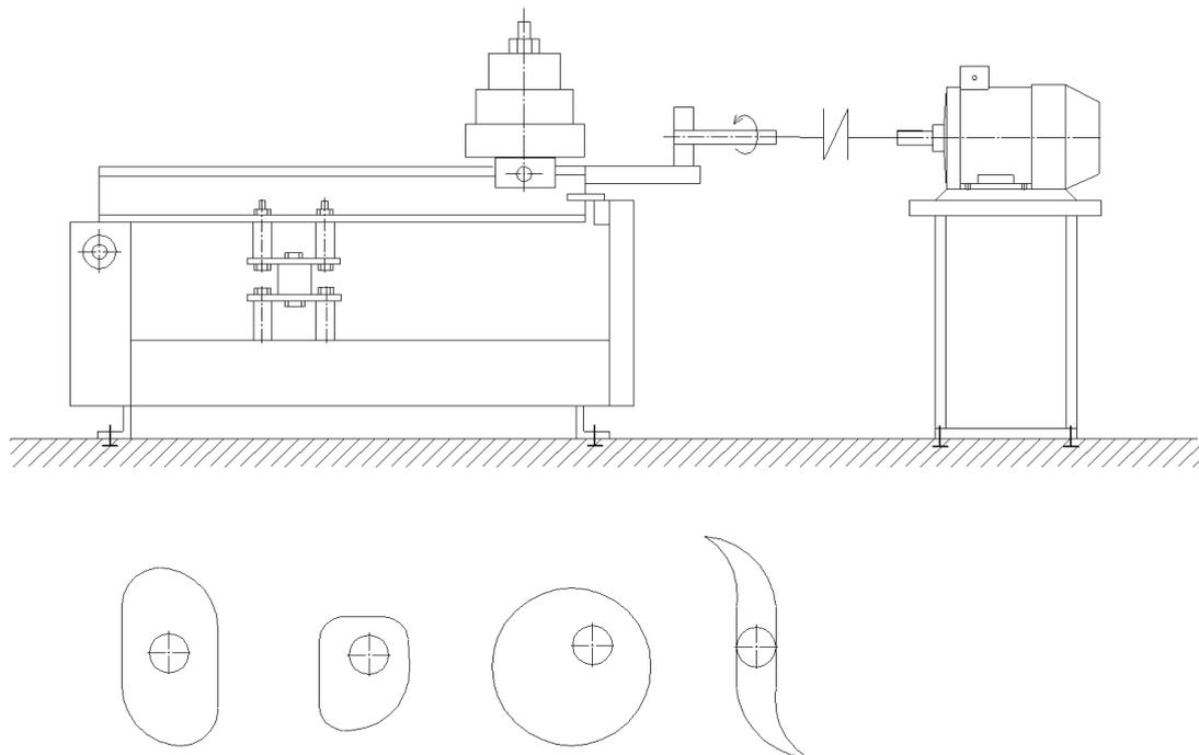
Fig. 6. Scheme of forced oscillations excitation system on the test bench by cam-eccentric mechanism
