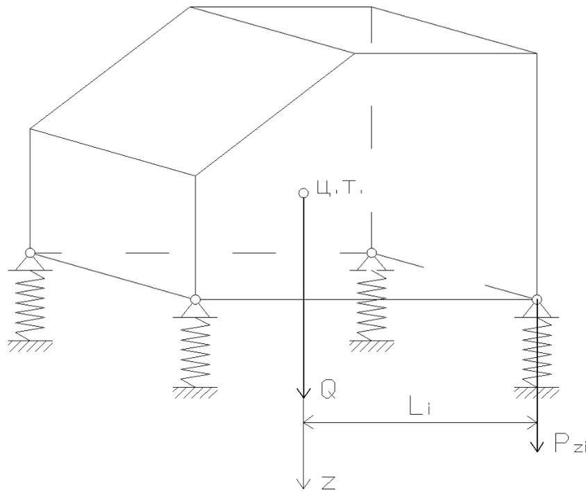
Fig. 4. Scheme of vibration isolators installation in the real technical object's suspension
