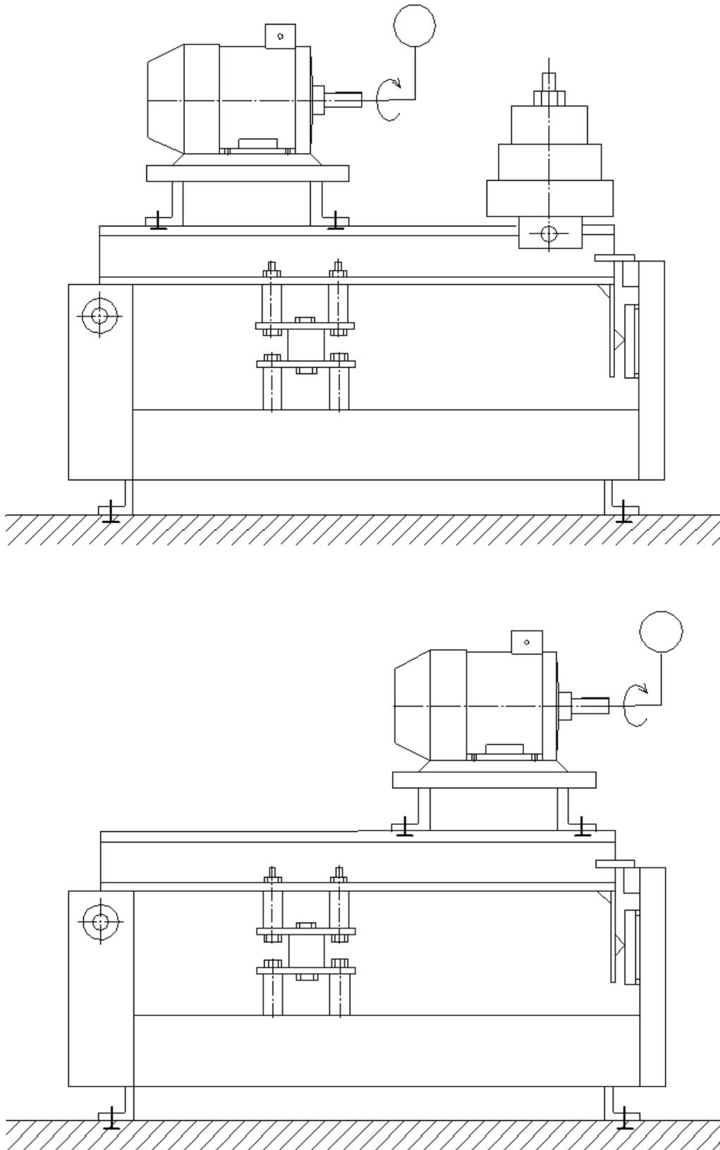
Fig. 7. Scheme of forced oscillations excitation system on the test bench by inertial exciter
