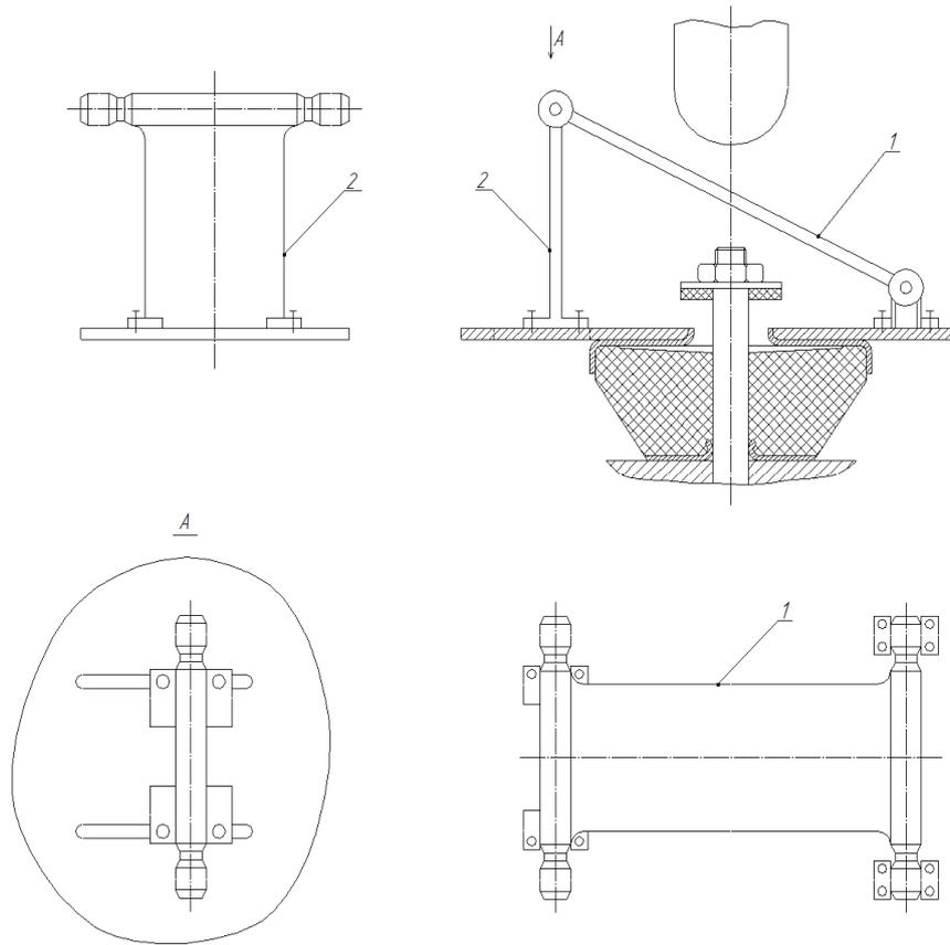
Fig. 5. Design of the device for loading the vibration isolator with vertical and lateral loads combination
