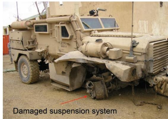
Fig. 1. Military vehicle "Cougar" after mine explosion [4]
