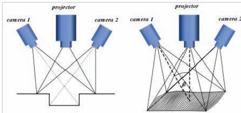
Fig. 2. Scanning using two cameras to increase scanning accuracy
