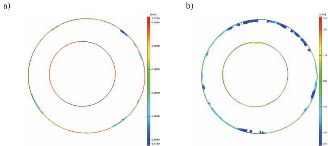
Fig. 8. Changes in profiles of the sidewall above the first ring, corresponding to the pistons in Fig. 7: a) the piston 7b, b) the piston 7c
