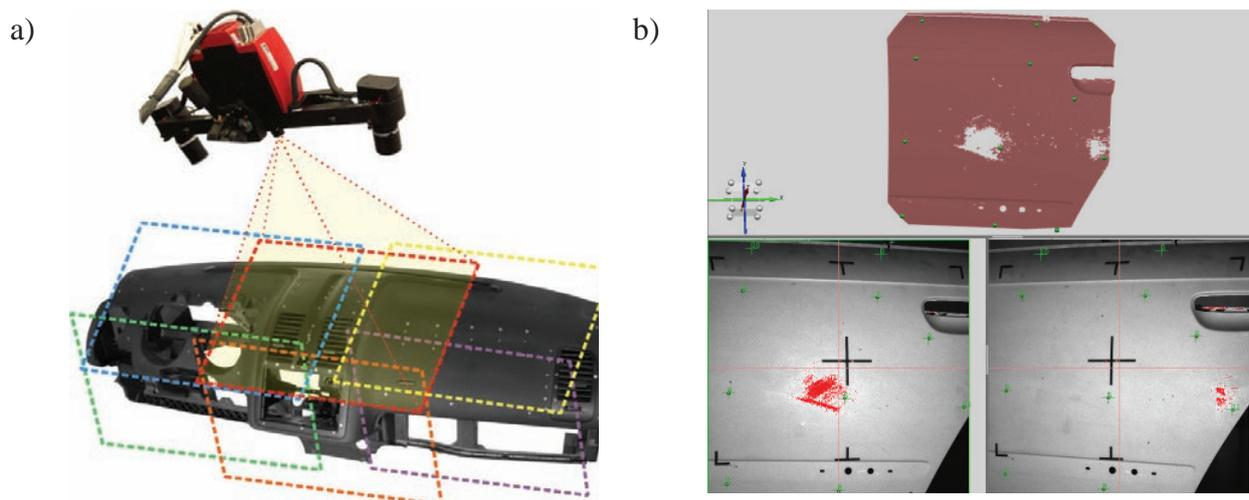
Fig. 4. Scan results: a) combining the surface images, b) discontinuity surface view of two cameras
