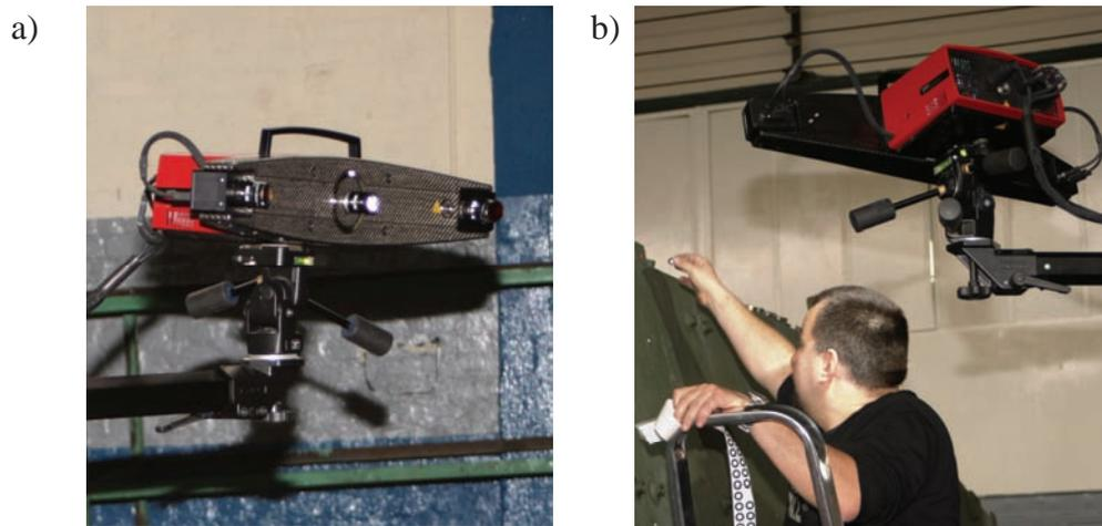
Fig. 3. Optical scanner: a) head of scanner with a projector and two cameras, b) sticking reference points on the scanned surface
