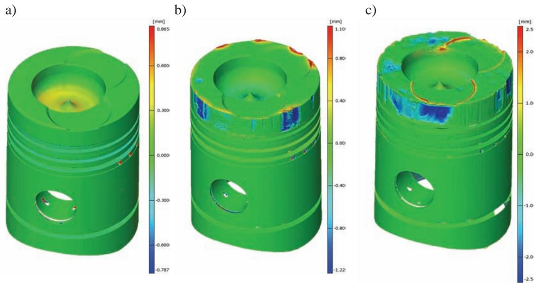
Fig. 7. The SW-680 engine piston: a) the new piston, b) the pistons damaged sides, c) damaged surface of the piston and piston head with burnouts
