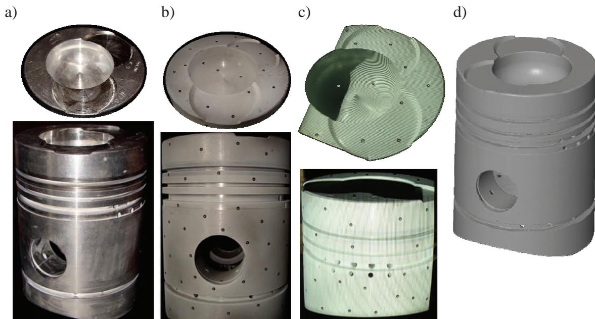
Fig. 6. Stages of piston scanning: a) prior to scanning, b) after tarnishing the surface and stick on reference points, c) illuminated by a projector during the scan, d) after the polygonization
