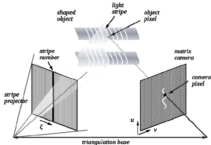
Fig. 1. Application of the triangulation principle in 3D scanning
