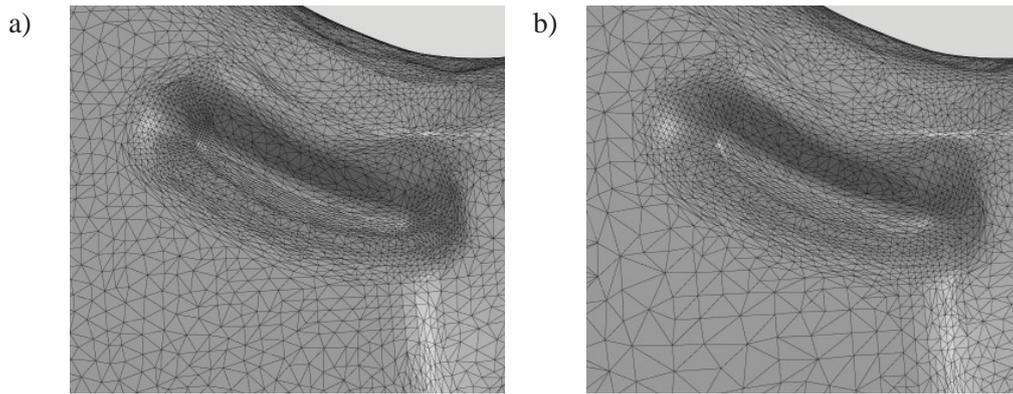
Fig. 5. Different grid density after polygonization, a) a dense grid, b) a rare grid
