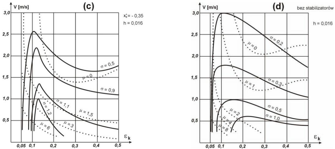
Fig. 2. Changes of the coefficient of damping and the degree of stability
