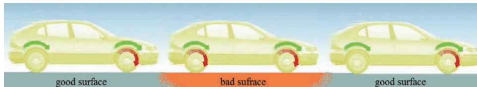
Fig. 4. The effect of the controller under varying conditions of adhesion: Green arrow – direction of rotation of the wheel, red arrow – wheel drive, bad road surface – a degraded surface properties, good surface - surface with good properties
