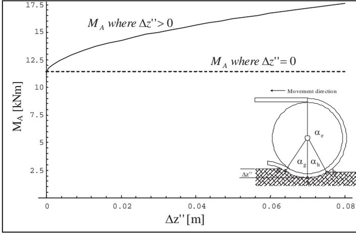
Fig. 6. Increase of driving moment  $M_A$  caused by wrap angle increase with additional angle  $\alpha_g = f(\Delta z'')$  [2]
