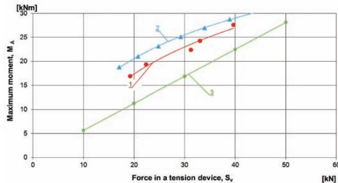
Fig. 3. Comparison of the results of measurements (1) with calculations based on: (2)-equation (7), (3)-Euler's law ( $\mu=0.8$ )[2]
