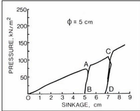
Fig. 4. Response of mineral soil for cyclic loading [9]
