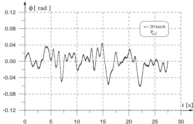
Fig. 9. Angular movements of the hull of the CV when driving through the ground
