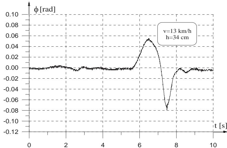
Fig. 7. Angular movements of the hull of the CV
