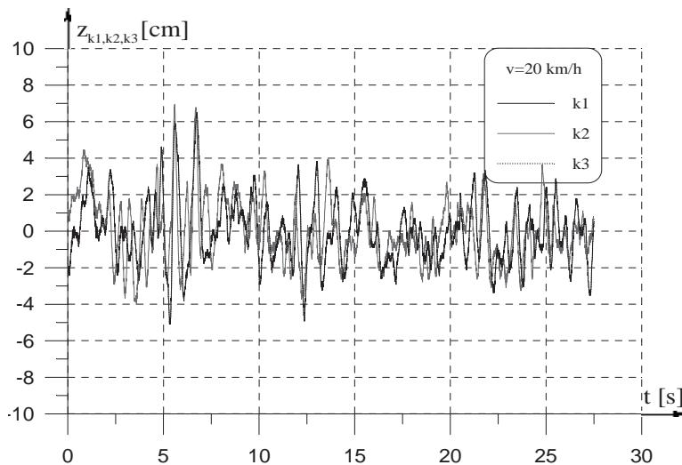
Fig. 10. Vertical displacements of carrying wheels when driving through the ground
