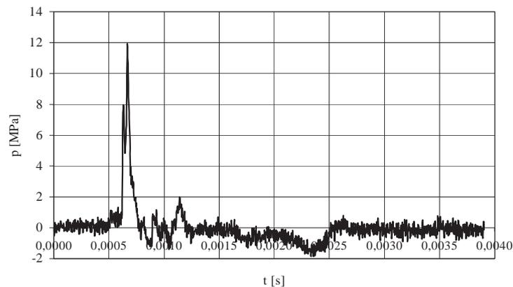
Fig. 13. Distribution of pressure acting on a selected area of the bottom of the hull
