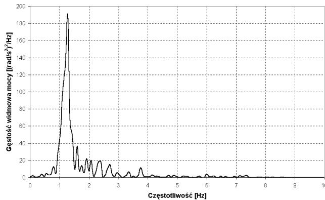
Fig. 15. Power spectral density estimator of longitudinal vibration of the hull tank
