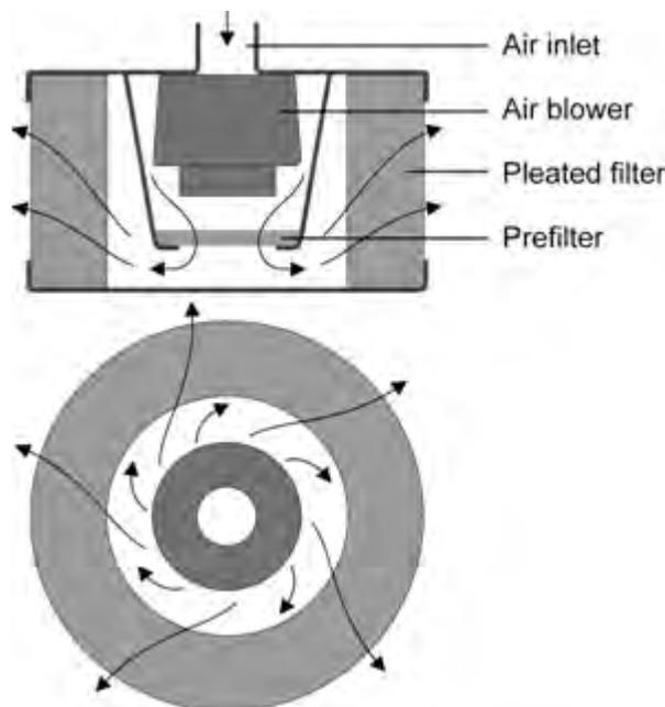
Fig. 3. Setup of the filter with integrated prefilter for coarse particles and blower
