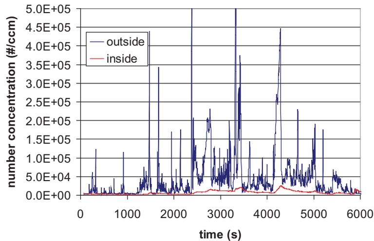
Fig. 17. Results using the nanocleaner filter
