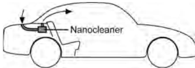
Fig. 6. One possible solution to mount the filter system
