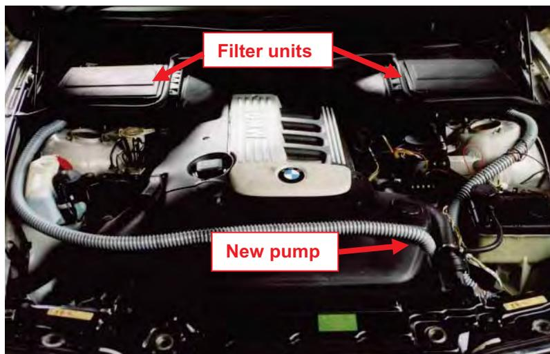
Fig. 15. The original filter of the BMW 530 has been replaced by high efficiency filters. Air is supplied by a blower, which is also placed in the engine compartment
