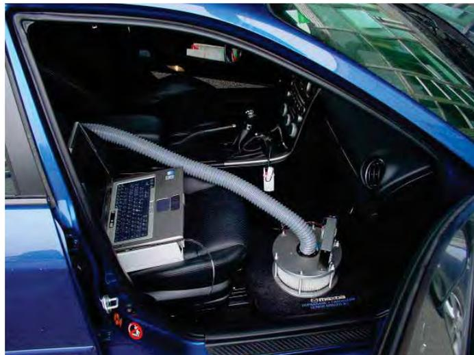
Fig. 7. Filter, particle sensor (below notebook) and Notebook for data acquisition
