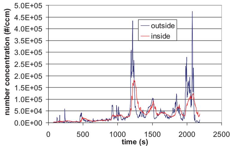
Fig. 16. Results with regular ventilation system
