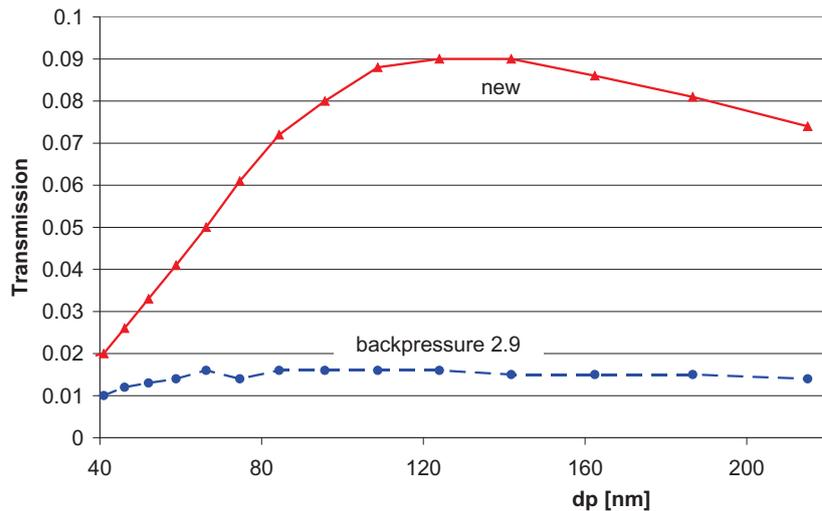
Fig. 2. Filter-efficiency: Transmission as function of particle size for the new filter and for the filter loaded to a pressure drop of 2.9 mbar
