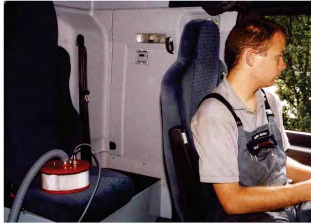
Fig. 11. Nanocleaner placed in a truck cabin. Two units are used for the test measurements
