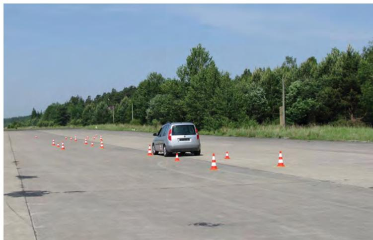
Fig. 1. Test VDA ISO TR 3888 – top view: track of the test (size in the meter), under view: Škoda Roomster during tests on the airport Hradčany-Mimoň
