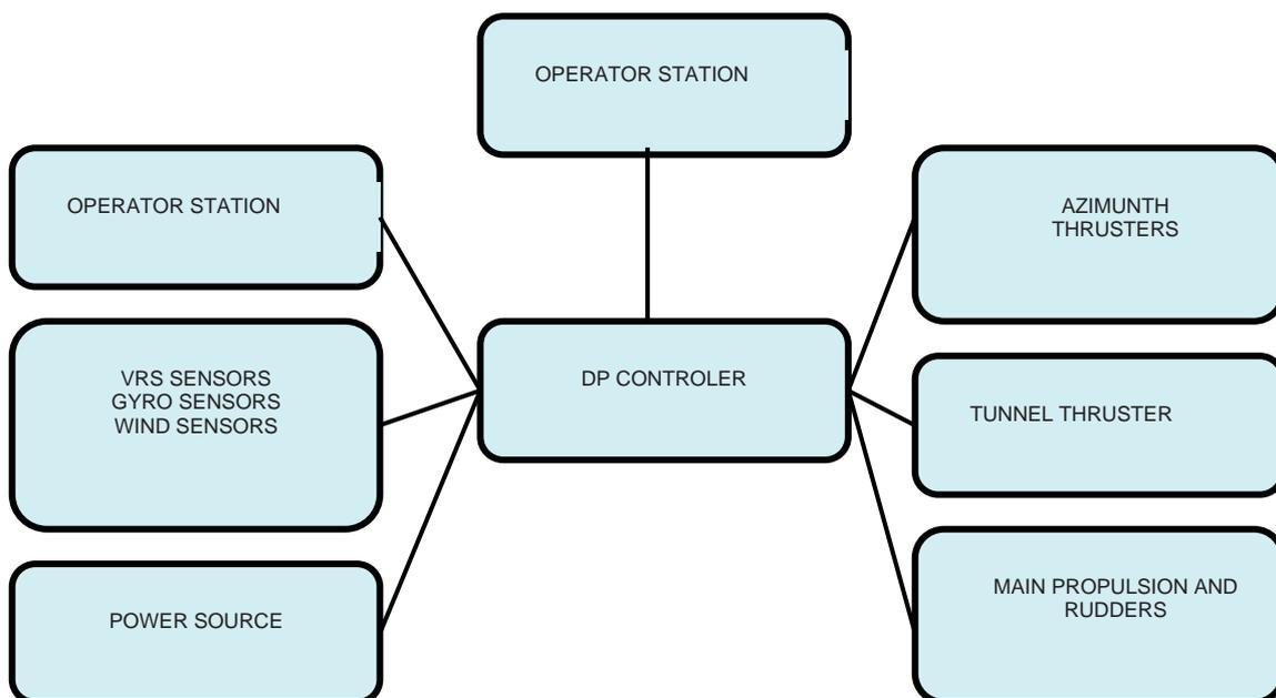
Fig. 10. Simplified scheme of DP system [9]
