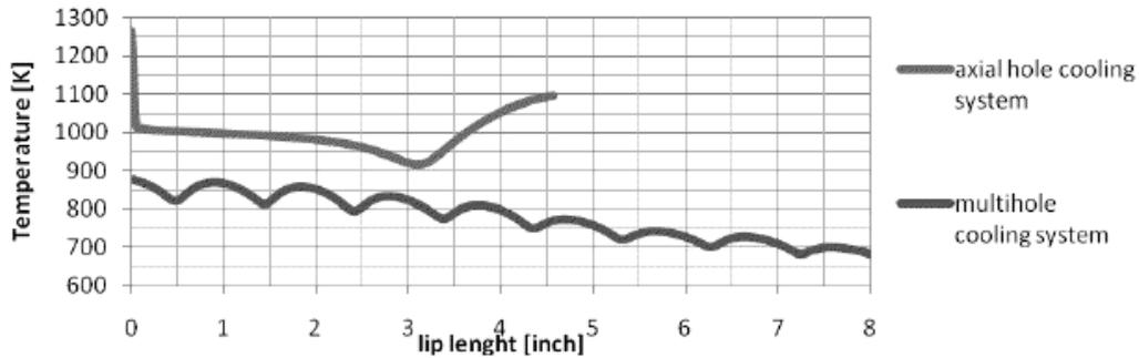
*Fig. 15. Temperature plots liner lip (from the hot side) - all cases*
