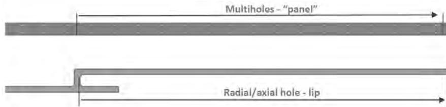
*Figure 16. Areas from which temperatures were read - liner panel (from the hot side)*
