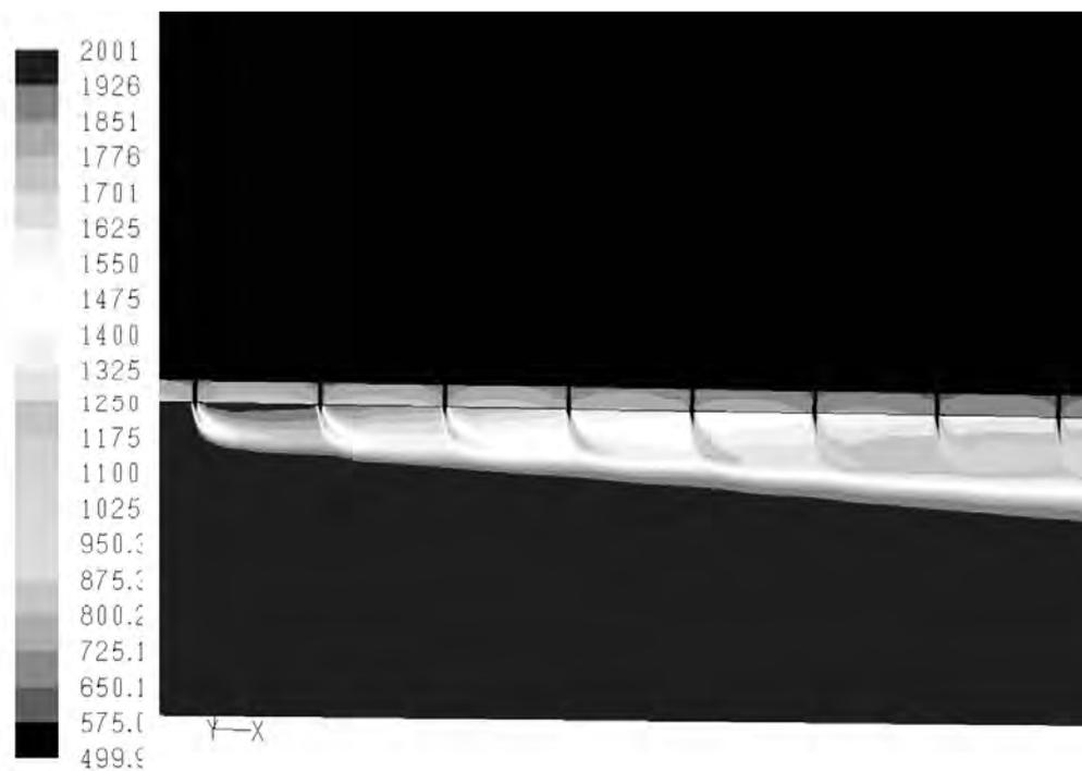
*Fig. 10. Final model multiholes cross-section temperature [up to 2000K]*
