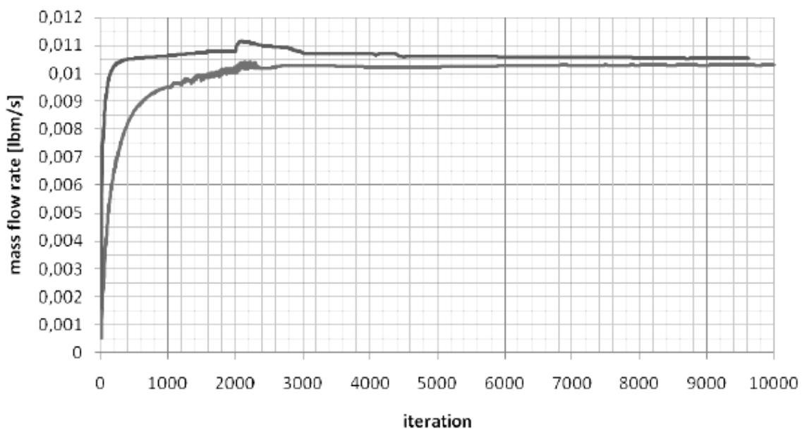
*Fig. 6. Comparison of mass flow rate for four different cooling systems*
