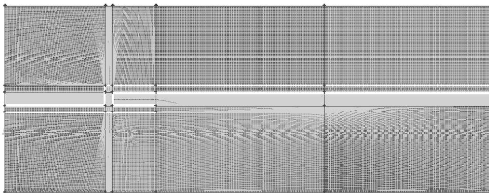
*Fig. 5. Axial hole cooling system mesh*
