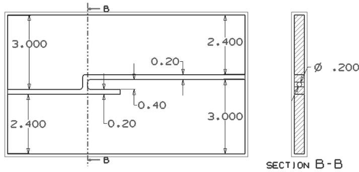
Fig. 1. Drawing of cooling slot with axial hole (All dimensions are in inches)
