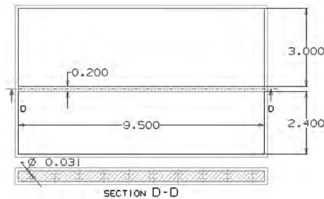
Fig. 3. Sketch of liner with multihole cooling holes (All dimensions are in inches)
