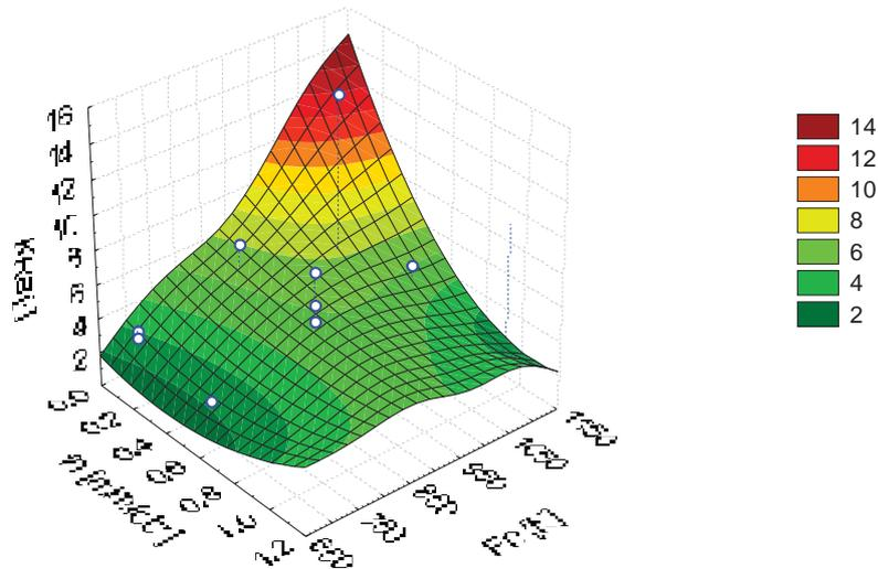
Fig. 1. Effect of burnishing feed and force on the  $K_{Ra}$  value  $K_{Ra}$  of Ni-5%Al coatings
