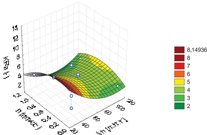
Fig. 2. Effect of burnishing speed and feed rate on the  $K_{Ra}$  value of Ni-5%Al coatings
