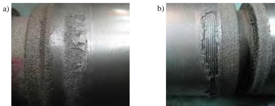
Fig. 4. Coatings surface ( $F_n = 1100$  N,  $f_n = 0.08$  mm/rev,  $V_n = 28.26$  m/min) [9]: a) Ni-5%Al after three burnishing, b) Ni-5%Al-15%Al<sub>2</sub>O<sub>3</sub> after a single burnishing
