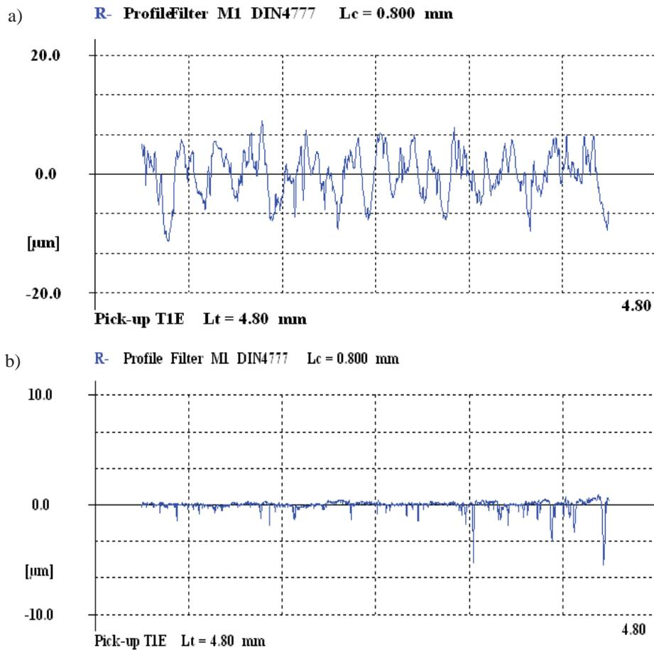
Fig. 5. Examples of coating roughness profiles of Ni-5%Al a) after turning , b) after burnishing
