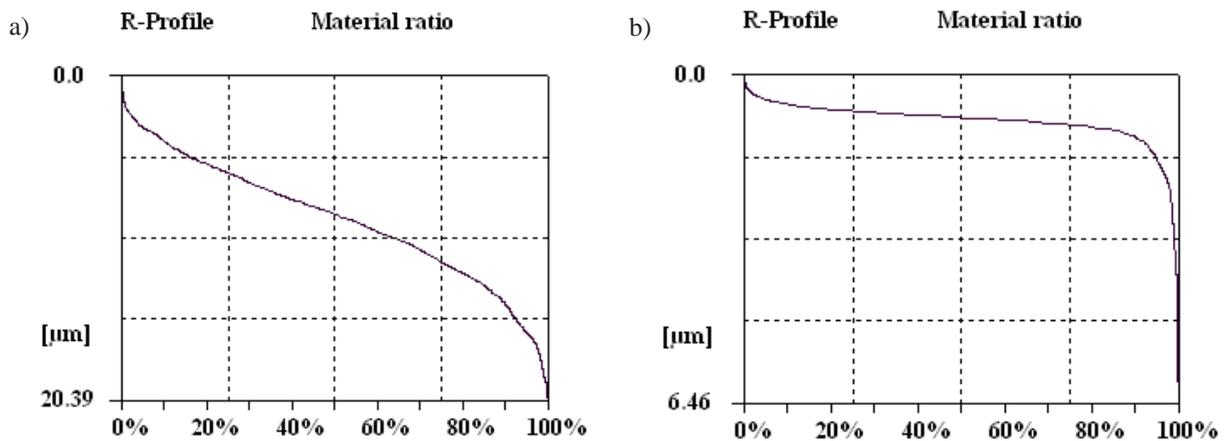
Fig. 6. Examples of material ratio curves of Ni-5%Al coating surface: a) after turning , b) after burnishing
