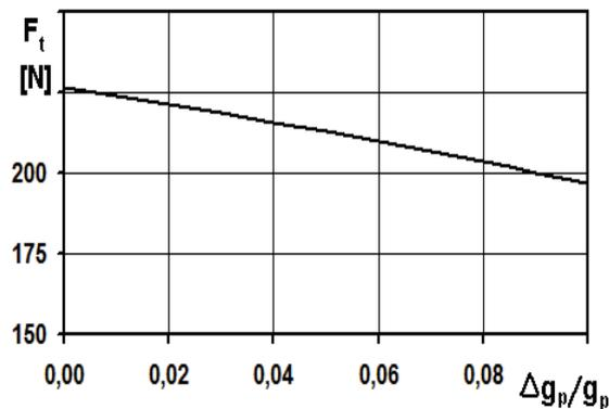
Fig. 9. The effect of relative drop in ring radial thickness  $\Delta g_p/g_p$  on value of tangential force  $F_t$  for ring diameter  $d = 480$  mm
