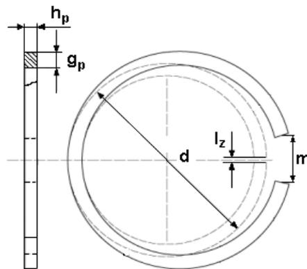
Fig. 2. A sketch of compression ring: free (continuous line) and mounted in bore (dashed line);  $d$  – bore diameter,  $g_p$  – ring radial thickness,  $h_p$  – ring axial height,  $m$  – free ring joint,  $l_z$  – joint gap
