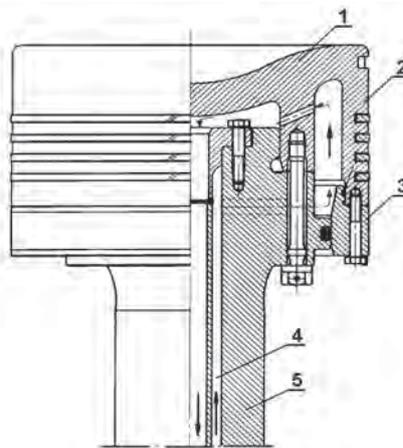
Fig. 1. A sketch of crosshead engine piston; 1 - crown, 2 - land, 3 - skirt, 4 - oil ducts, 5 - piston rod
