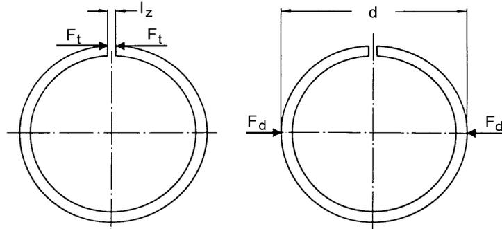
Fig. 4. A sketch of ring with locations of tangential  $F_t$  and central  $F_d$  force measurements points
