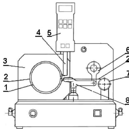
Fig. 5. Test rig for measurements of ring elasticity: 1 – piston ring, 2 – clamping band, 3 – measurement plate, 4 – dynamometer measuring axle, 5 – dynamometer, 6 – vibrator, 7 – reel, 8 – eccentric lever [2]
