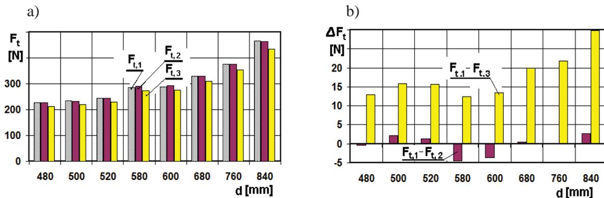
Fig. 7. Comparison of ring tangential force  $F_t$  carried out on a test sample of marine engine rings;  $F_{t,1}$  – value given by producer,  $F_{t,2}$  – value obtained for  $K = 13.31$  and  $F_{t,3}$  – value obtained for  $K = 14.14$  (a) and arrangement of differences in this force (b)
