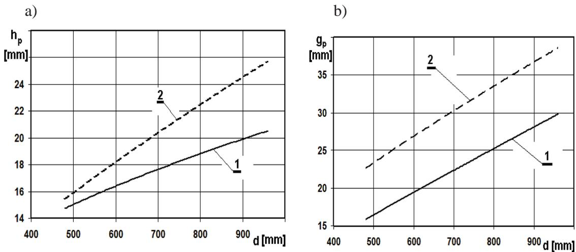
Fig. 3. Relations between ring diameter  $d$  and its: a – axial height  $h_p$ ; b – radial thickness  $g_p$ ; presented results have been achieved for a group of marine engine piston rings: modern – 1 (continuous line), previous – 2 (dashed line)
