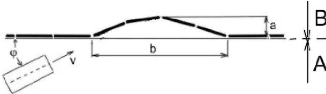
Fig. 1. The following quantities describe such displacement:  $a$  - maximum lateral displacement,  $b$  - length of the active (movable) section of the barrier,  $\beta$  - angle of vehicle approach to the barrier with velocity  $v$
