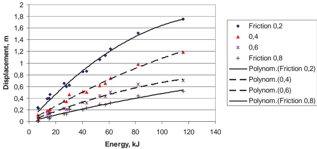
Fig. 5. Maximum Barrier Displacement vs. Impact Energy
