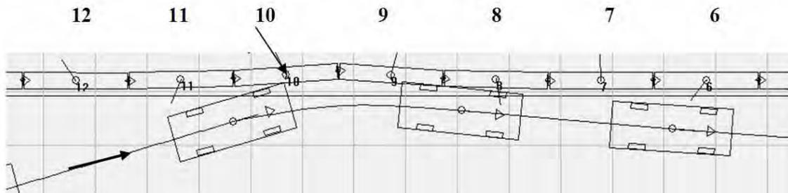
Fig. 4. The position of the barrier hit by the vehicle at a 16 degrees angle, vehicles centre of inertia trajectory and vehicle contours at 0.5 s intervals. The visible part of the barrier consists of segments 6-12
