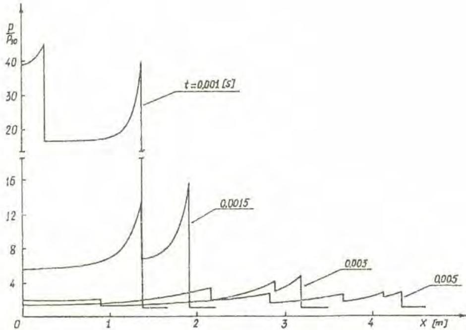
Fig. 9. The pressures distribution on the construction surface in the function of distance from the explosion epicenter, charge – 8 kg, channel height – 0.5 m
