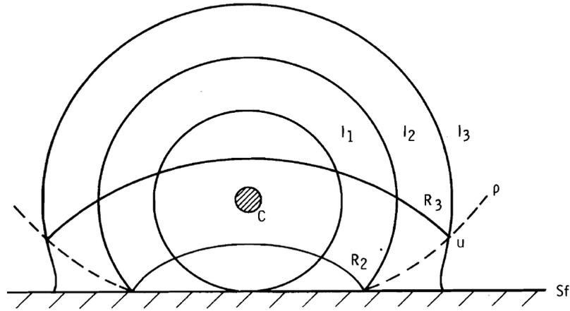
Fig. 4. Reflection of waves generated by detonation of strong charges from a rigid obstacle [7]
