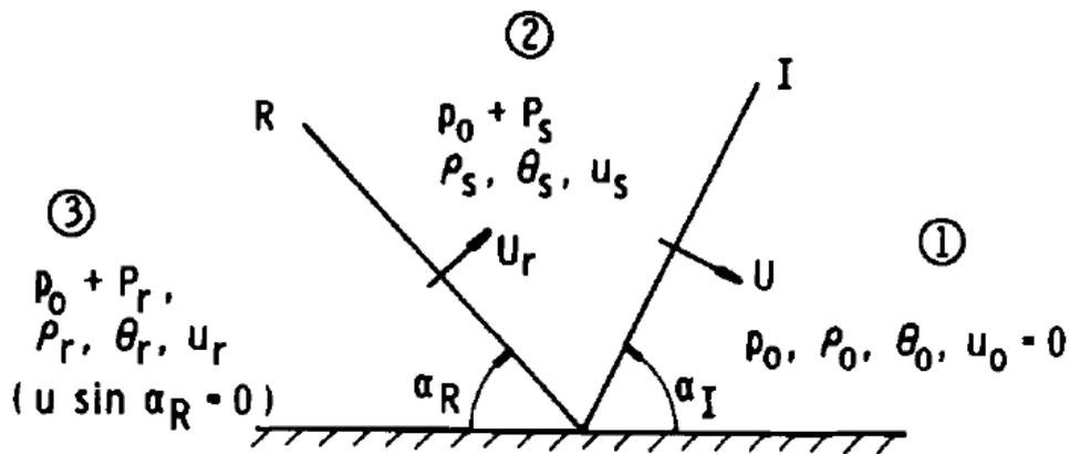
Fig. 3. The wave configuration near the wall in the scope of regular reflection [7]
