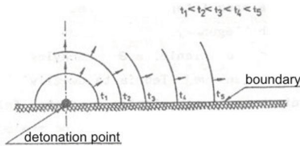
Fig. 1. Initial pressure wave originated as the result of the explosive material detonation [6]
