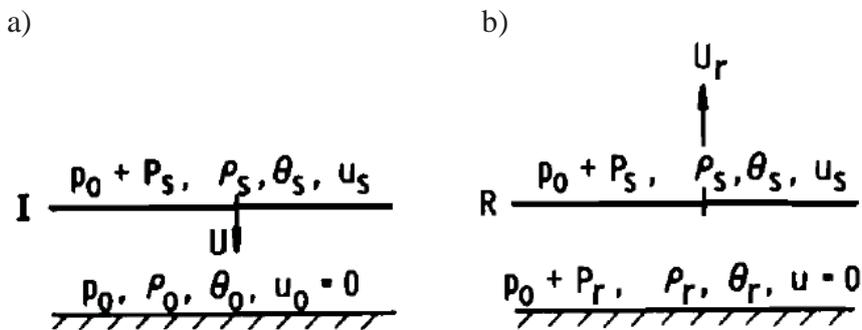
Fig. 2. An example of reflection of a flat wave falling on the stiff obstacle
