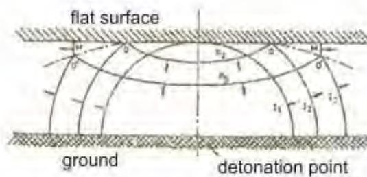
Fig. 6. The reflection of a spherical blast wave from a flat surface [6]
