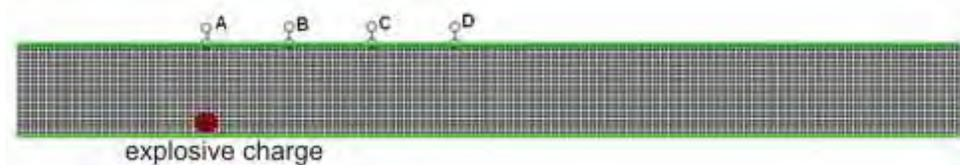
Fig. 10. A draft of a numerical model of a considered example. Green thick lines designate the surfaces limiting the gases outflow. Points A, B, C, D designate Euler cells in which the pressure values were charted
