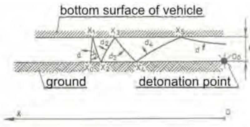
Fig. 8. The fronts of the subsequent blast waves
