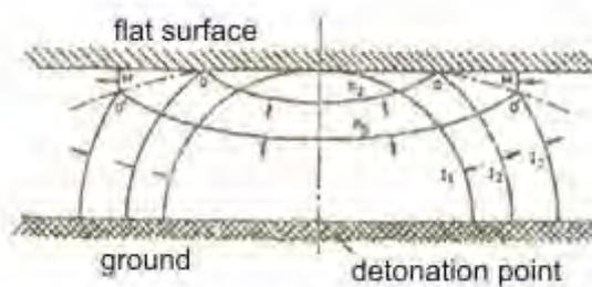
Fig. 6. The reflection of a spherical blast wave from a flat surface [6]
