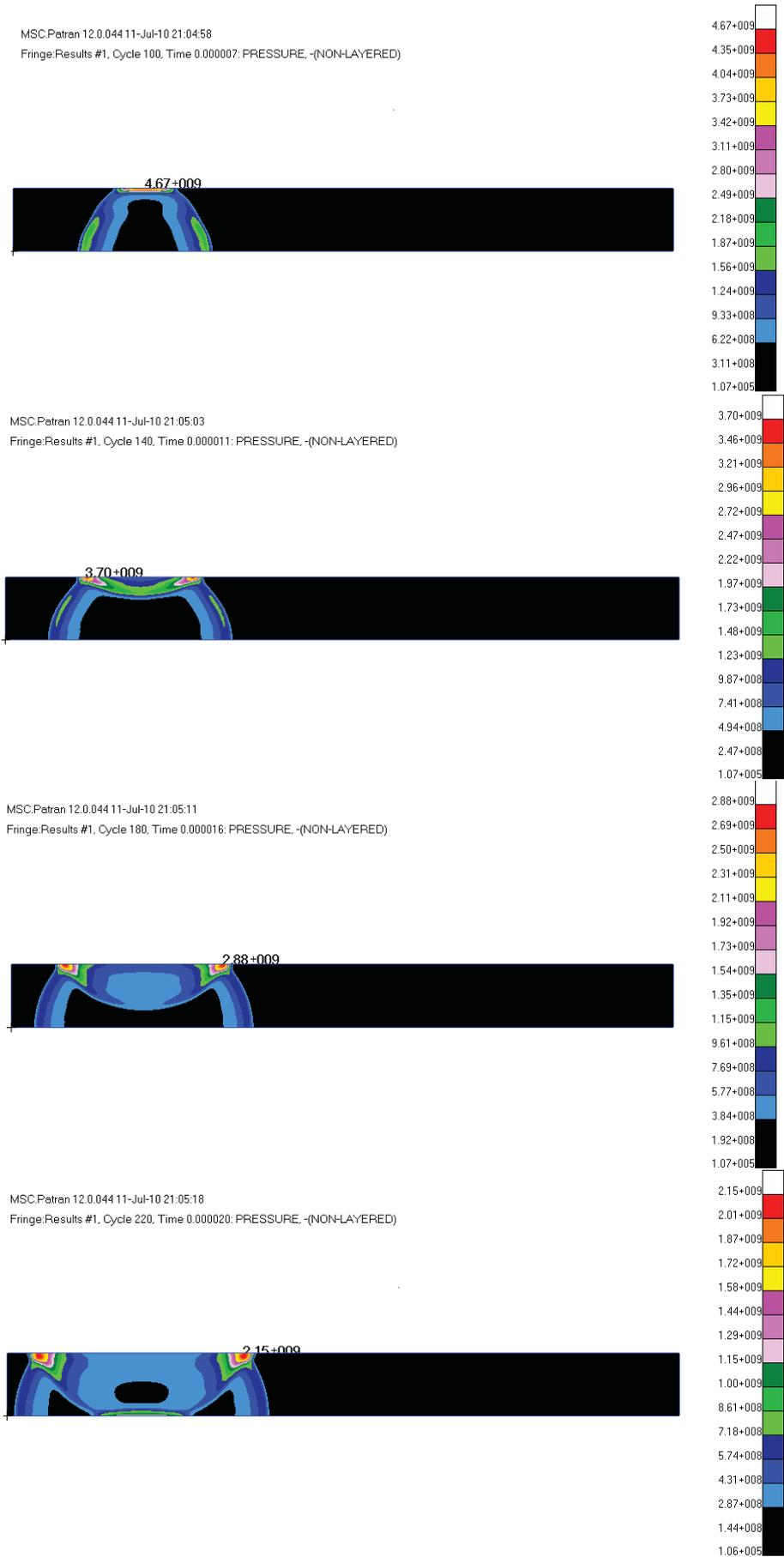
Fig. 12. Strengthening of the pressure impulse reflected from the upper wall and the further wave propagation
