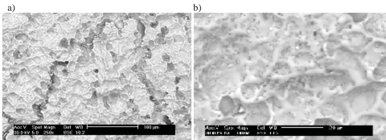
Fig. 4. Characteristic area of the surface layer of heat resistant nickel alloy ŽS6K-WI after casting and laser ablative cleaning - apparent micro partial melting zones
