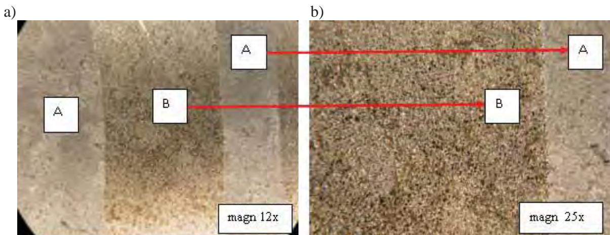
Fig. 6. Jet engine turbine blade made (cast) of nickel based alloy WI ŻS6K purified by the use of the laser: A - greasy surface, B - purified surface by the use of the radiation of pulsed Nd: YAG laser with power density  $q = 1.53 \cdot 10^6$  W/cm<sup>2</sup>, and scanning speed  $v = 5$  m / s
