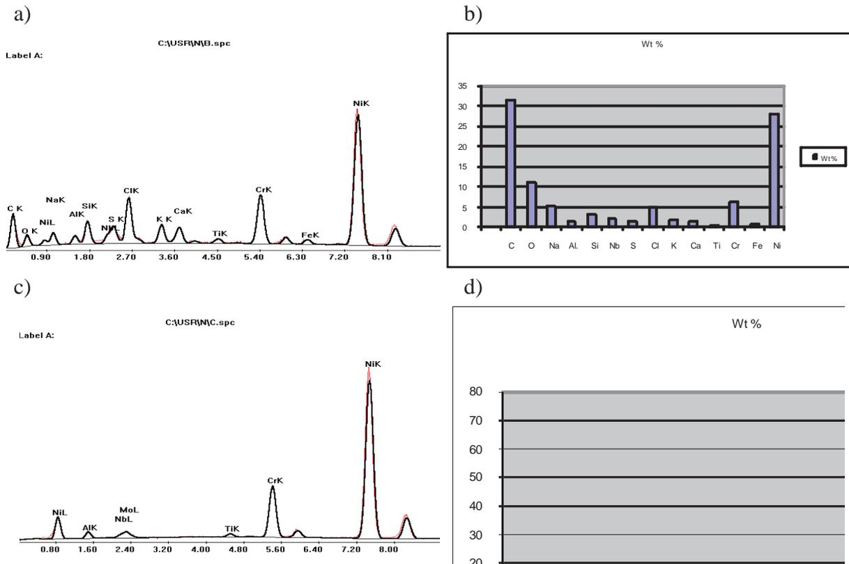
Fig. 5. The tests results of chemical constitution in the characteristic micro-zones of surface layer of high-temperature creep resisting nickel alloy: a, b - in the state after casting, c, d in the state after casting and laser cleaning
