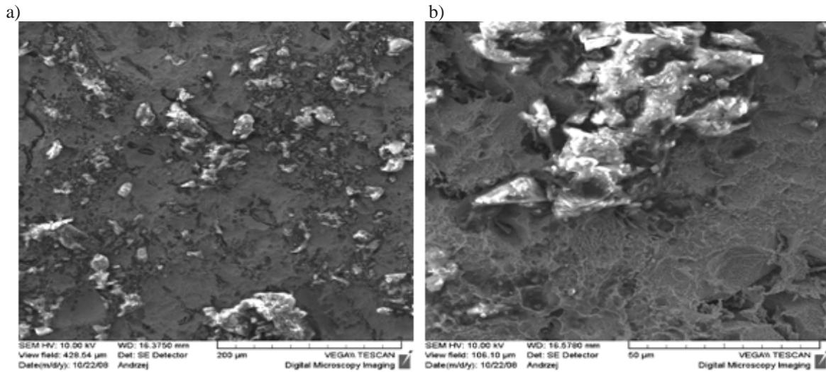
Fig. 2. The characteristic surface topography of heat resistant nickel alloy ZS6K-WI used in the manufacture of turbine blades of aircraft engines - the material after casting
