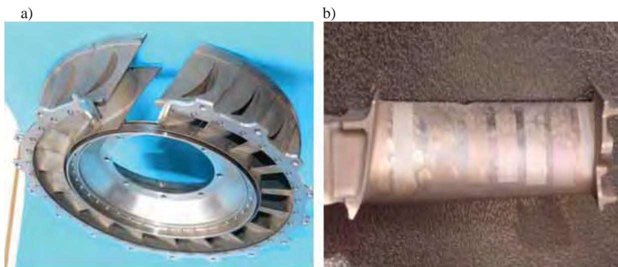
*Fig. 1. The studied elements of aircraft turbine engine: a) the turbine blades before cleaning, b) turbine blade laser-cleaned in the laboratory conditions*
