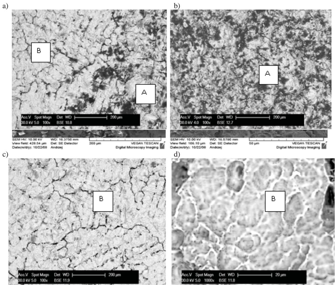
Fig. 3. Characteristic area of the surface layer of heat resistant nickel alloy ZS6K-WI after casting and laser ablative cleaning: A - a zone before cleaning, B - a zone after cleaning
