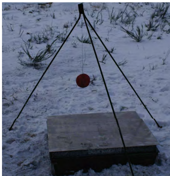
Fig. 11. The general view of a stand for testing the panels loaded with huge explosive charges
