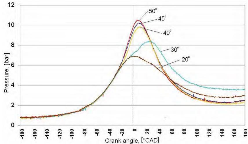
Fig. 6. Comparison of pressure courses in RCM combustion chamber for different ignition advance angles:  $20^\circ$  CAD,  $30^\circ$  CAD,  $50^\circ$  CAD BTDC (System configuration  $V_{kv}=10\%$ ,  $d=3$  mm, ignition in prechamber centre)
