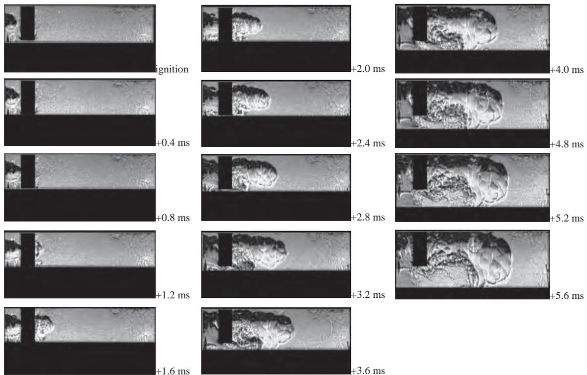
Fig. 2. Course of combustion in RCM for system configuration:  $V_{kw}=10\%$ ,  $d=3mm$ , ignition in the prechamber centre,  $\varphi_{wz}=20^\circ$  CAD BTDC
