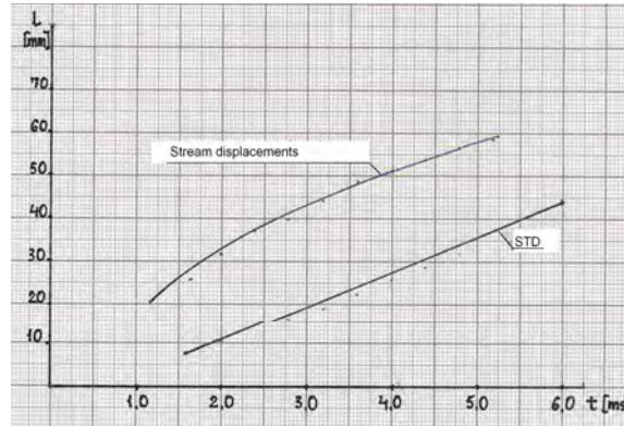
Fig. 3. Flame front travel versus time for the situation presented on fig. 2
