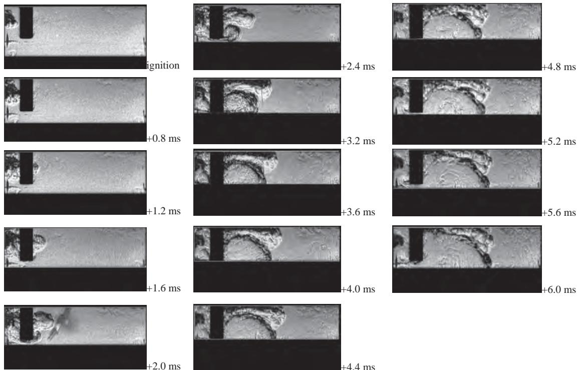
Fig. 4. Course of combustion in RCM for system configuration:  $V_{kw}=10\%$ ,  $d=3\text{ mm}$ , ignition in the prechamber centre,  $\varphi_{wz}=50^\circ \text{ CAD BTDC}$
