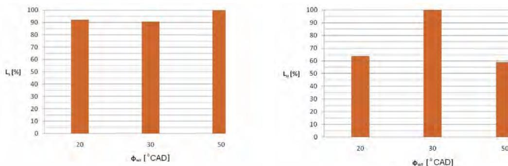
Fig. 7. Comparison of compression work ( $L_s$ ) and effective work ( $L_u$ ) of RCM for ignition advance angle:  $20^\circ$  CAD,  $30^\circ$  CAD,  $50^\circ$  CAD BTDC (System configuration  $V_{kv}=10\%$ ,  $d=3$  mm, ignition in prechamber centre)
