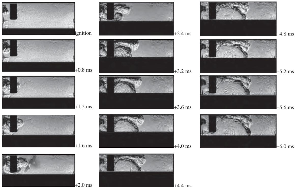
Fig. 4. Course of combustion in RCM for system configuration:  $V_{kv}=10\%$ ,  $d=3\text{mm}$ , ignition in the prechamber centre,  $\varphi_{wz}=50^\circ$  CAD BTDC
