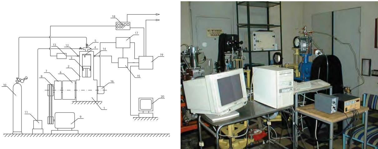
*Fig. 1. Schematic and view of RCM test stand*
