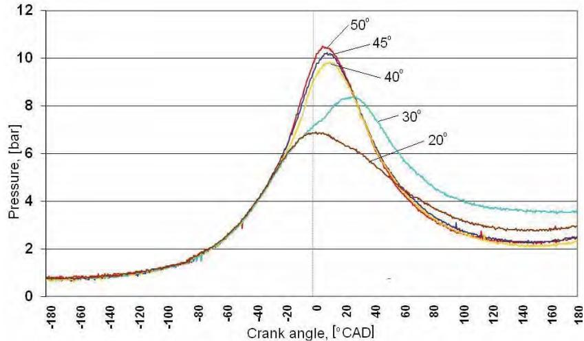
*Fig. 6. Comparison of pressure courses in RCM combustion chamber for different ignition advance angles: 20° CAD, 30° CAD, 50° CAD BTDC (System configuration  $V_{kw}=10\%$ ,  $d=3$  mm, ignition in prechamber centre)*
