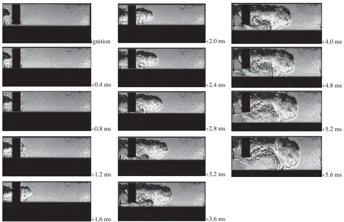
Fig. 2. Course of combustion in RCM for system configuration:  $V_{kw}=10\%$ ,  $d=3\text{mm}$ , ignition in the prechamber centre,  $\varphi_{wz}=20^\circ \text{ CAD BTDC}$
