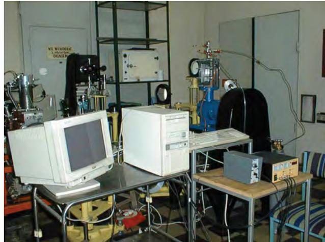
*Fig. 1. Schematic and view of RCM test stand*
