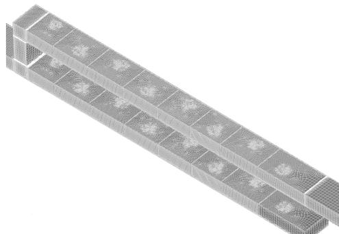
Fig. 10. Impingement cooling system mesh
