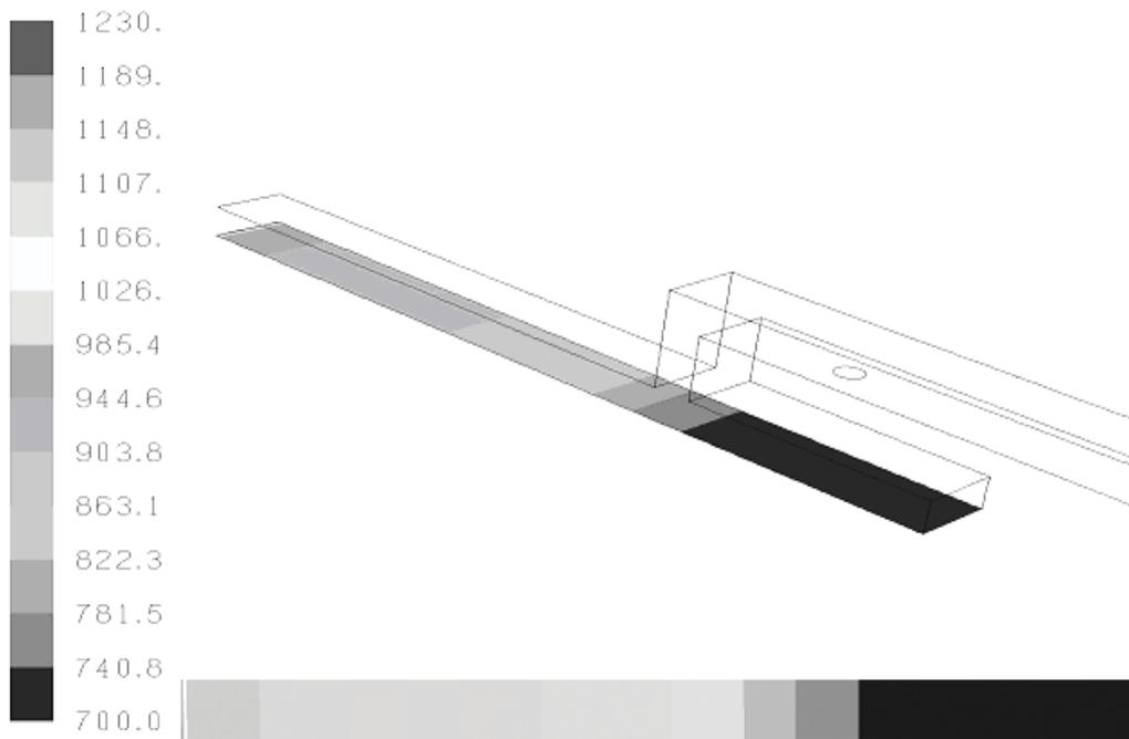
Fig. 15. Temperature layout on the liner lip – radial hole cooling
