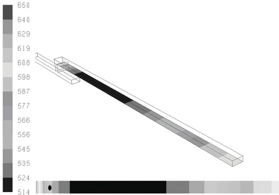
Fig. 13. Temperature layout on the liner panel – radial hole cooling
