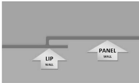
Fig. 12. Heat loaded combustor areas
