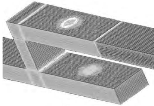
Fig. 9. Radial hole cooling system mesh
