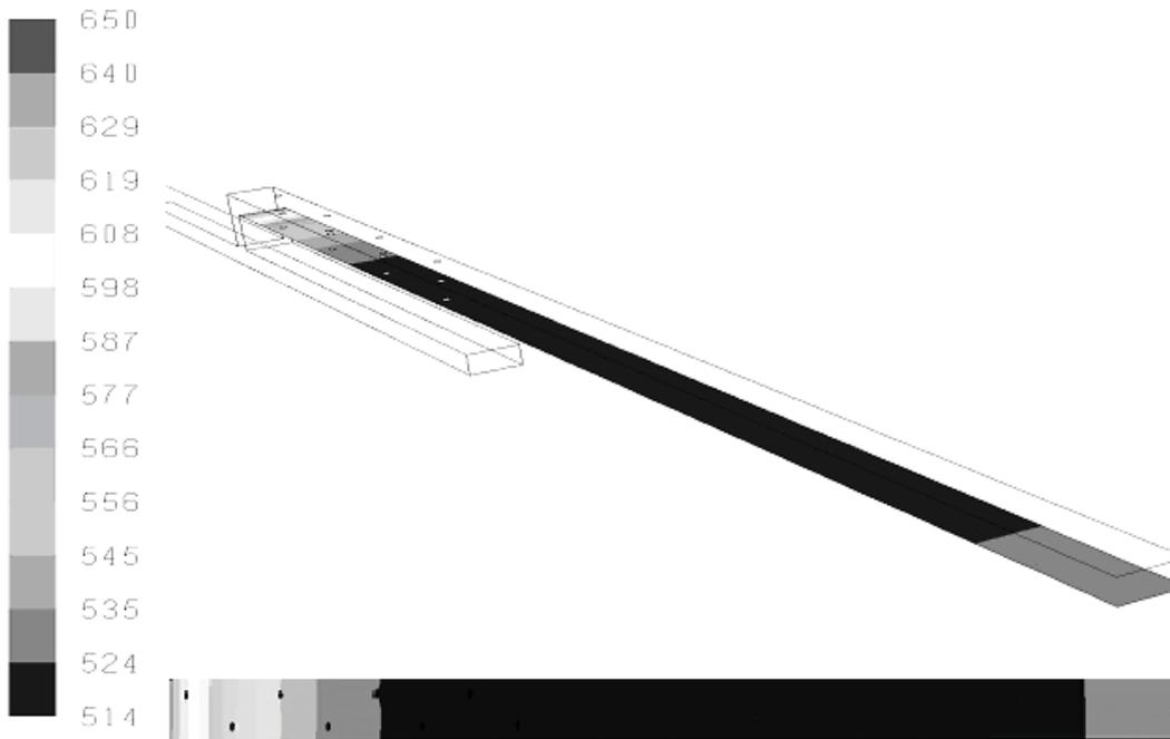
Fig. 14. Temperature layout on the liner panel – impingement cooling
