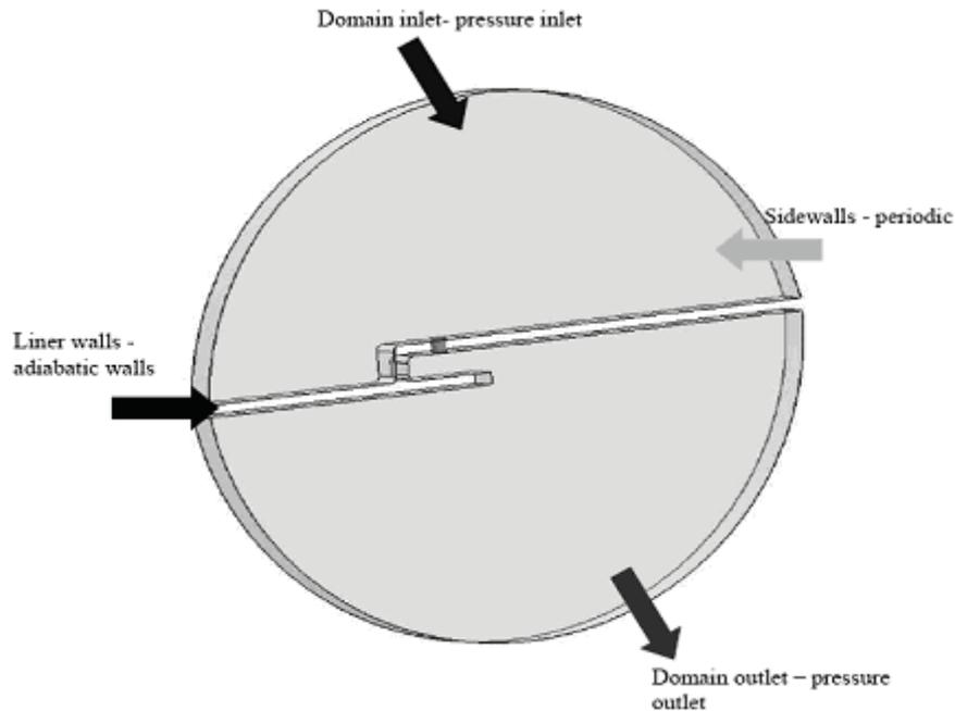
Fig. 5. Flowcheck model boundary conditions
