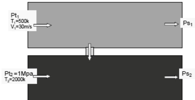
Fig. 11. Boundary conditions preliminary setting
