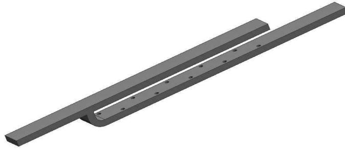
Fig. 2. Cooling slot with impingement cooling
