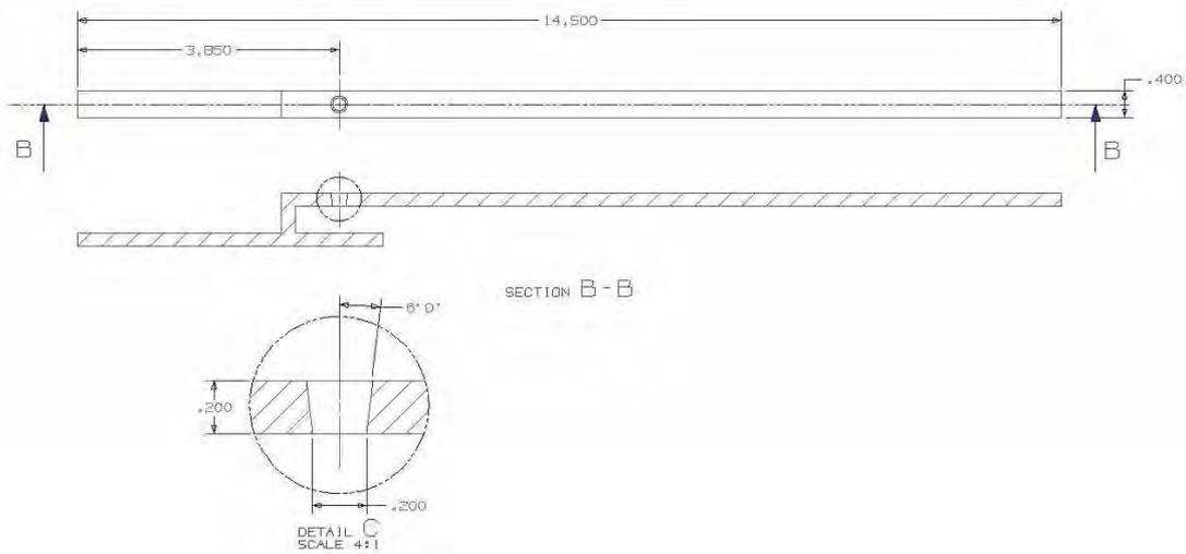
Fig. 7. Analyzed geometry - radial hole details
