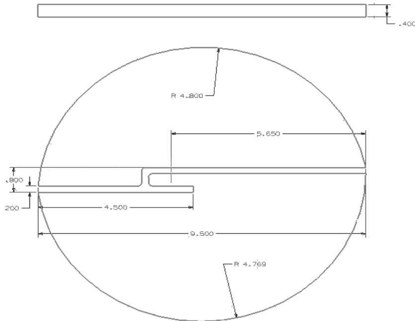
Fig. 3. Flowcheck model geometry details
