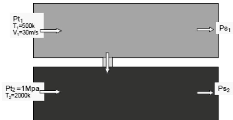
Fig. 11. Boundary conditions preliminary setting
