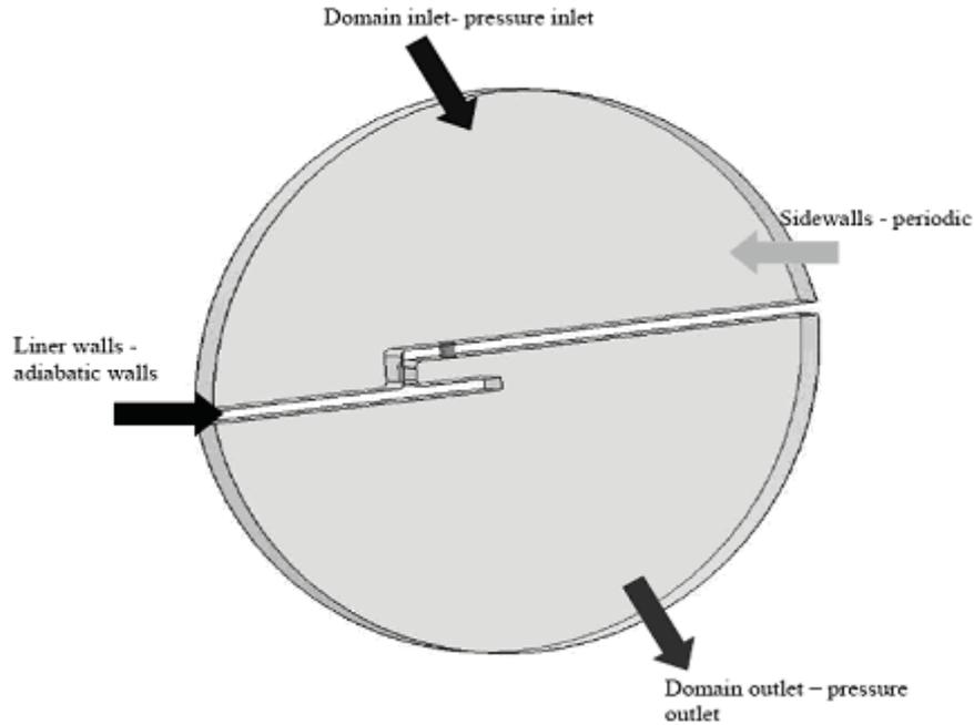
Fig. 5. Flowcheck model boundary conditions
