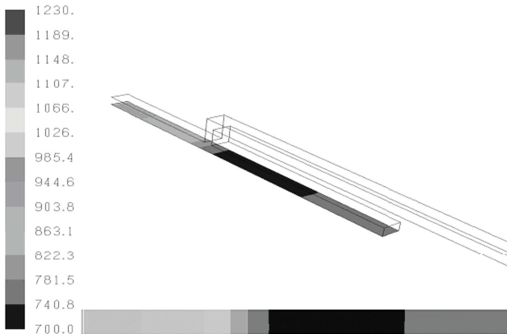
Fig. 16. Temperature layout on the liner lip impingement cooling
