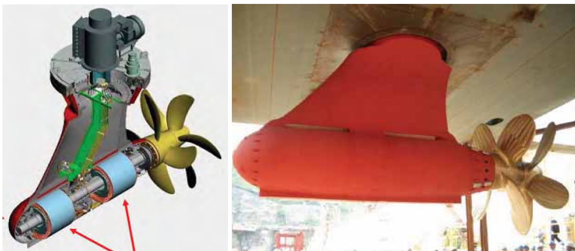
Fig. 3. Contra-rotating pod propellers with two shafts and two electrical motors [5]
