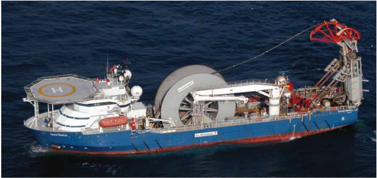
Fig. 1. Pipe laying vessel „Seven Mavica” [www.subsea7.com]
