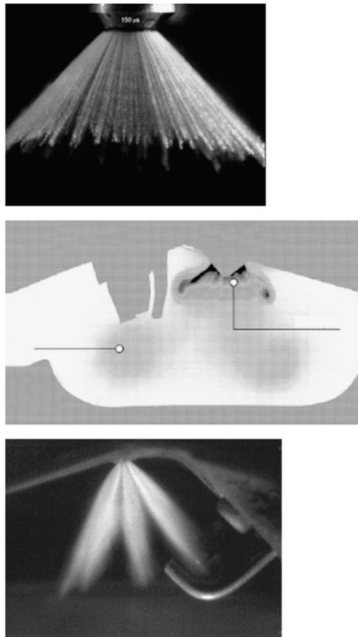
Fig. 2. Spray- and spray/spark-plug imaging for SGDI engines: from the top: near-injector-tip spray imaging of a piezoelectric outwardly opening pintle injector and MIE scattering image of a multihole injector spray
