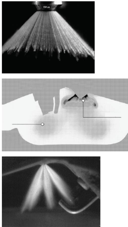
Fig. 2. Spray- and spray/spark-plug imaging for SGDI engines: from the top: near-injector-tip spray imaging of a piezoelectric outwardly opening pintle injector and MIE scattering image of a multihole injector spray
