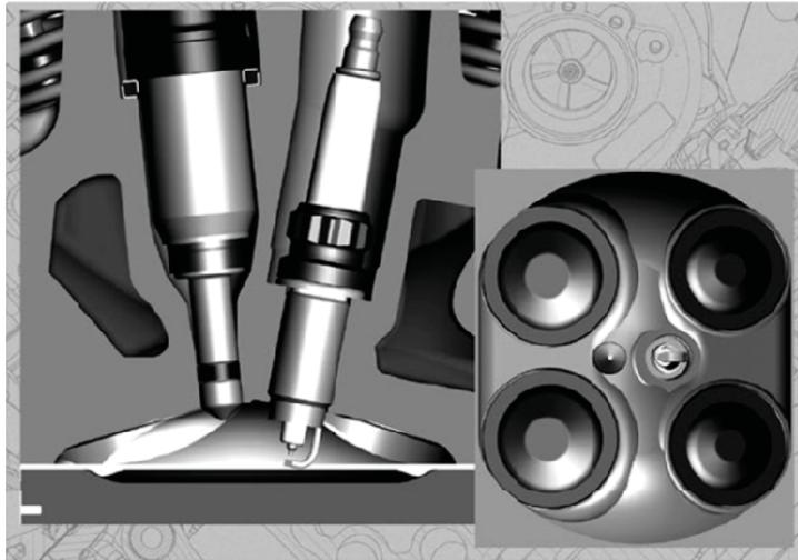
Fig. 1. Combustion chamber SGDI engine
