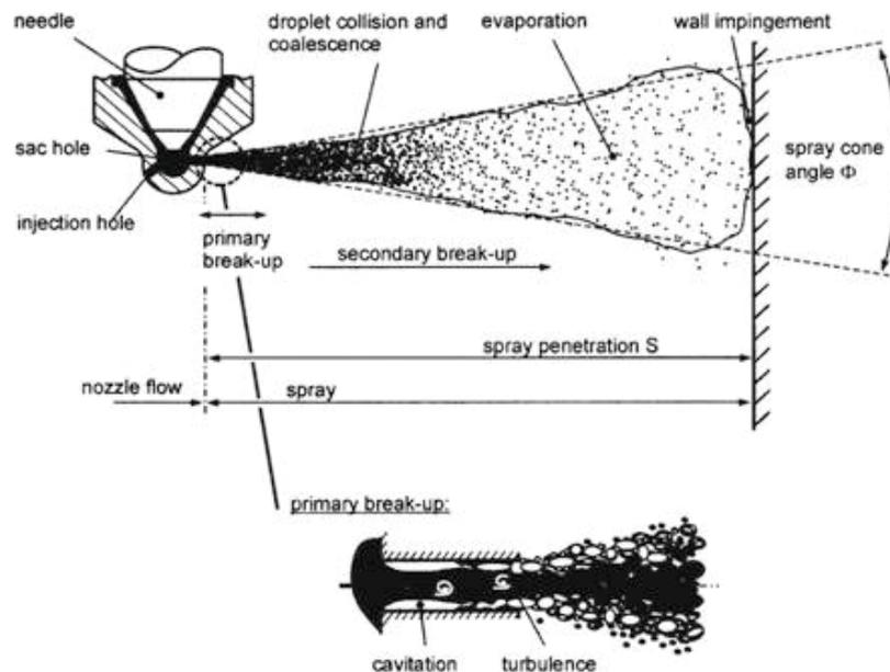
Fig. 3. Different flow regimes in high pressure diesel spray [Reitz,1994]
