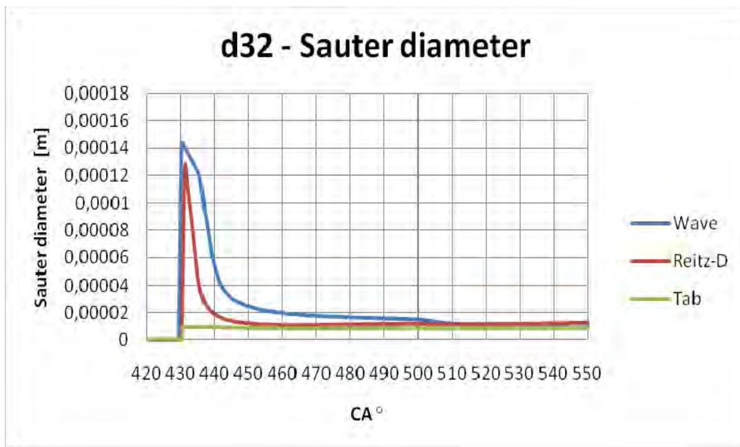
Fig. 8. SMD diameters as a result of different breakup models
