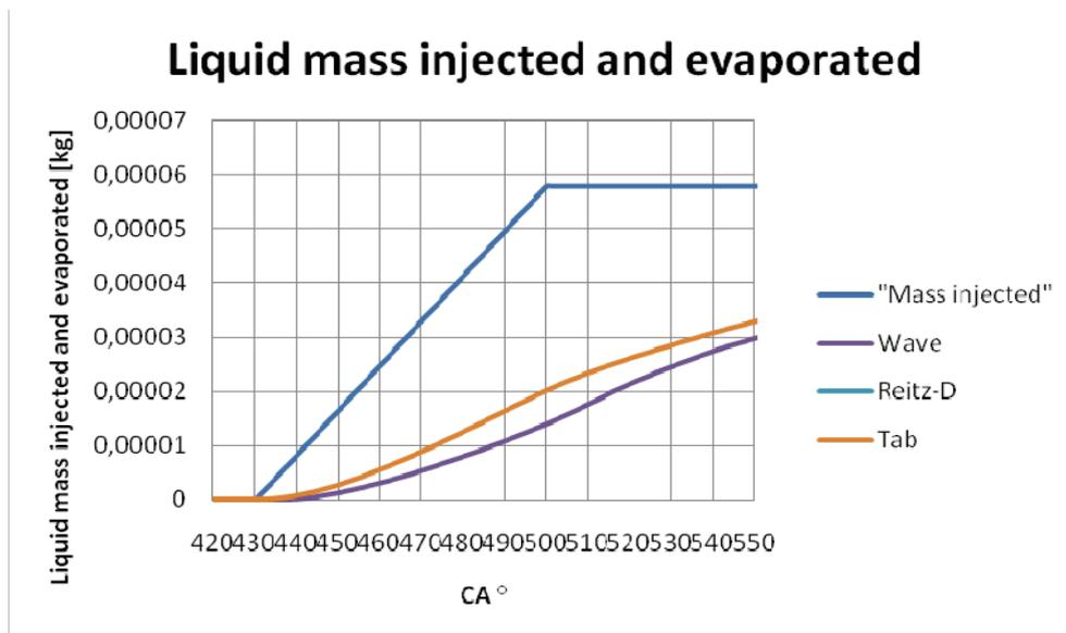
Fig. 10. Simulated fuel mass injected and evaporated
