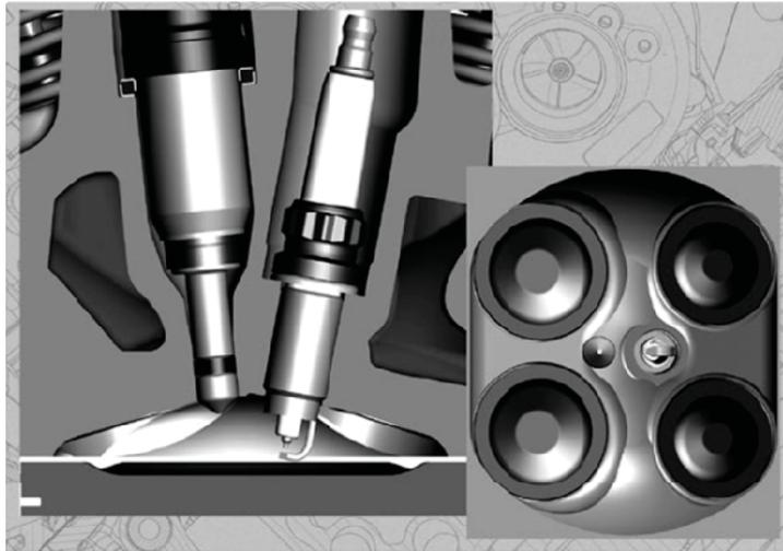
Fig. 1. Combustion chamber SGDI engine
