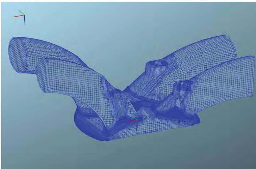
*Fig. 5. Mesh model from 340 to 360 CA*
