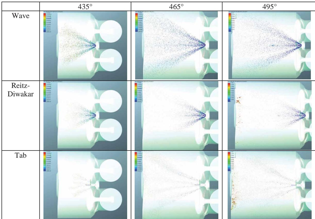
Comparison of simulated SMD diameter (Fig. 8) penetration (Fig. 9) and mass evaporated (Fig. 10) has been presented. It can be seen from these figures that smallest SMD diameter result for TAB model what is not correct in compare with another breakup models and even to experimental results for n-heptane [1]. The experimental results for injected ethanol with multi hole GDI injectors are still not available.
