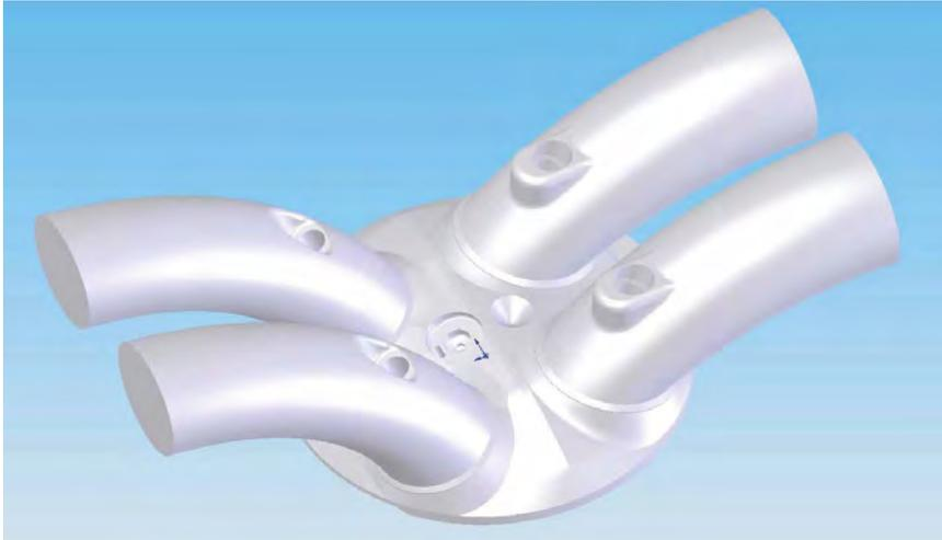
*Fig. 4. 3D model for BMW engine cylinder with inlet and outlet channels*
