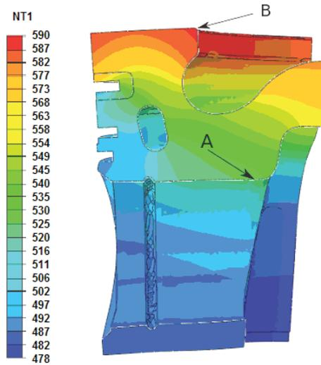
Fig. 5. Computed temperature distribution ( $p_e=1.772\text{ MPa}$ ,  $n=1600\text{ 1/min}$ ). Point B indicates the mesh node in which the temperature reaches the highest value in presented cross-section
