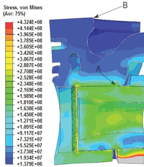
Fig. 6. Von Mises stress and their accumulation in mesh node market with the letter A ( $p_e=1.772\text{ MPa}$ ,  $n=1600\text{ 1/min}$ )
