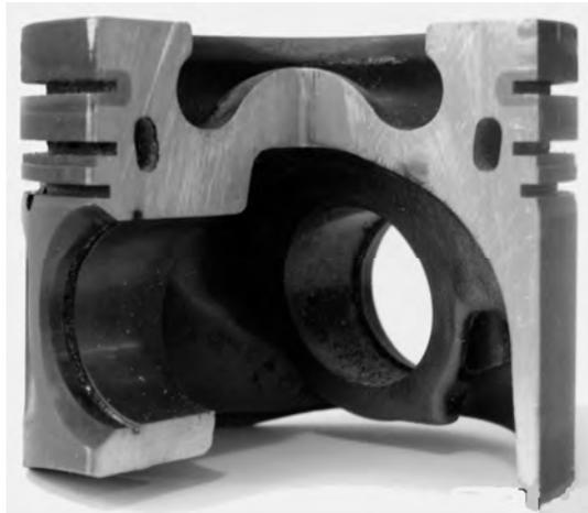
*Fig. 2. Cross-section of piston being the analysis object. The cooling channel and carrier of the top sealing ring are shown*
