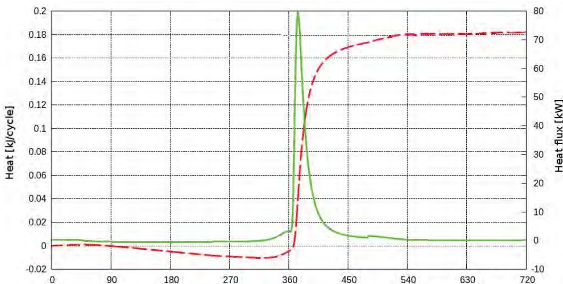
Fig. 4. Heat loses for piston (dashed line) and instantaneous heat flux for piston surface being with contact with working medium (solid line) as example results of engine cycle modelling done in SILNIK program ( $p_e=1.64$ MPa,  $n=3500$  1/min)
