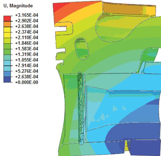
Fig. 8. Total deformation of hot piston loaded by mass forces, pressure and non uniform temperature field
