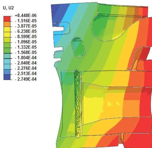
Fig. 7. Radial deformation of the hot piston decrease piston clearance to 0.05mm at the external edge of piston crown
