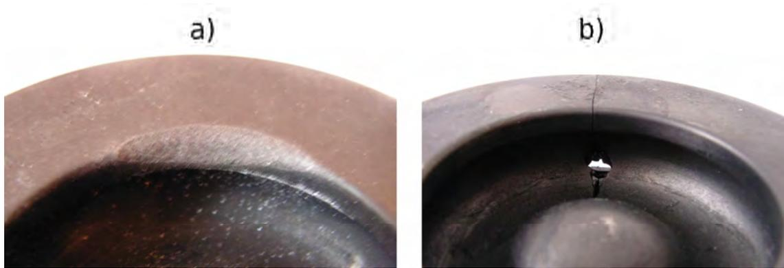
Fig. 1. Examples of failures typical for pistons of modern diesel engines: a) erosion of piston crown acted directly by burning spray of fuel , b) perforation and rupture of piston crown
