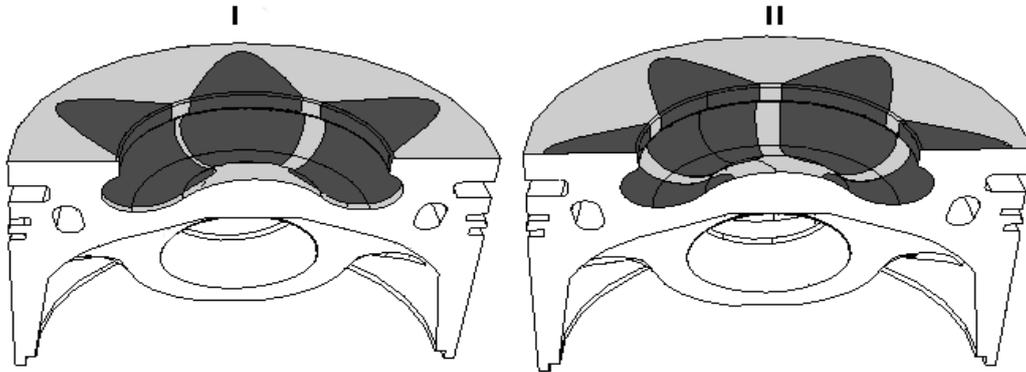
Fig. 3. Two computation cases determined by injector position against piston crown: I- burning fuel injected by injector acts piston area above the hub, II- piston hub area located between two fuel sprays
