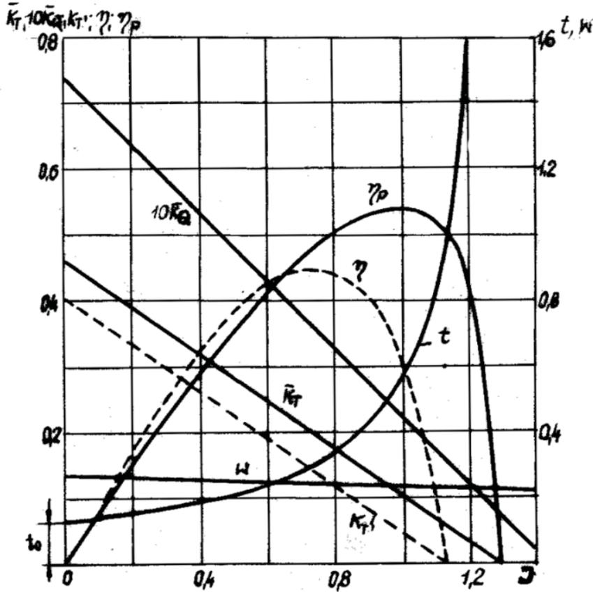
Fig. 1. Characteristics of a propeller working behind a hull of a vessel where:  $K_T$  - thrust coefficient,  $K_Q$  - torque coefficient,  $\eta_p$  - efficiency of an idle propeller,  $t$  - suction coefficient,  $w$  - wake fraction,  $\eta_h$  - efficiency of a propeller working behind a hull
