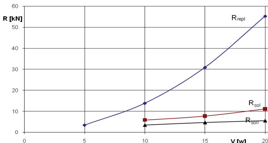
Fig. 5. Resistance of dragged propellers 1- locked, 2- freewheeling- I approximation, 3- freewheeling- II approximation
