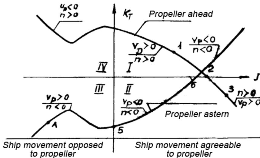
Fig. 2. Universal characteristics of a propeller for  $H/D = idem$
