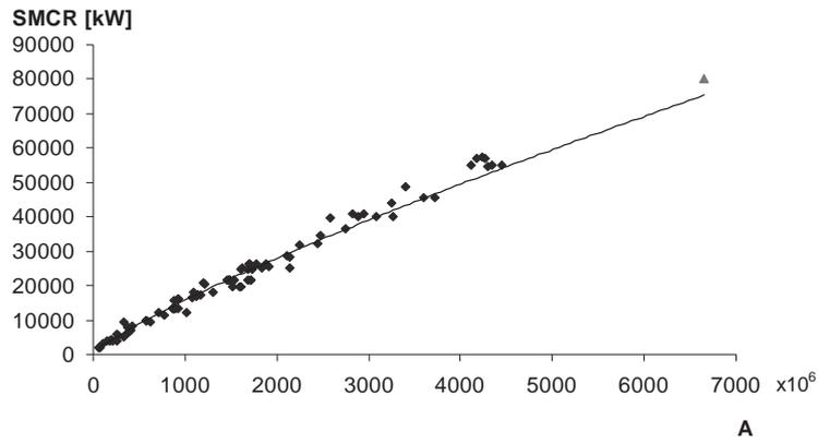
Fig. 5. Specified Maximum Continuous Rating and function A exponent relation
