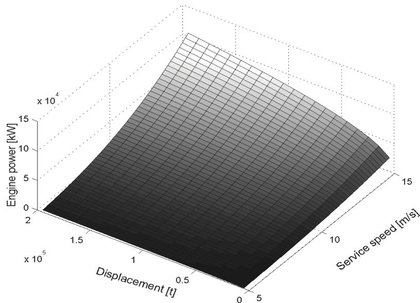
Fig. 6. Relation between Specified Maximum Continuous Rating, displacement and speed of the sea going ship
