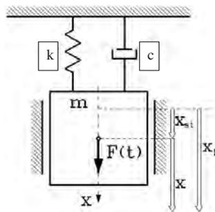
Fig. 1. System model of 1 degree of freedom
