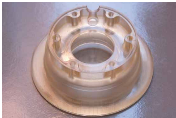
Fig. 4. Prototype SLA after UV irradiation (prepared for the final stage of cleaning and polishing the surface)
