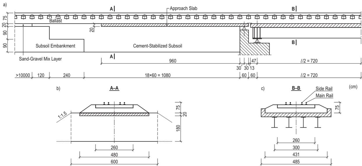
Fig. 3. The modernized ballasted track in the KNI 140070 bridge area: a) a longitudinal section; b) a cross-section in the approach zone; c) a cross-section over the bridge span
