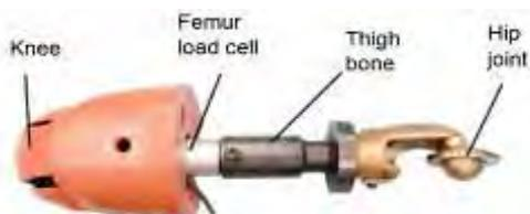
Fig. 3. Force transducer in the dummy's femur
