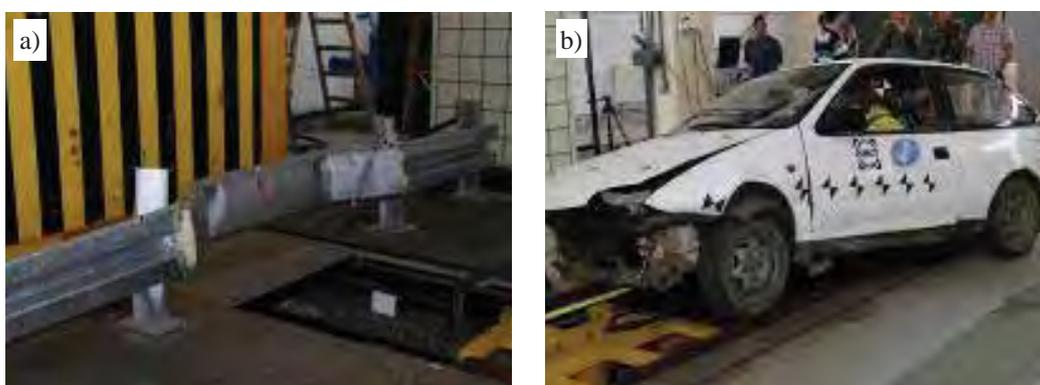
Fig. 8. Deformation of the tested protective road barrier type 1B (a) and Suzuki Swift car's deformation (b)
