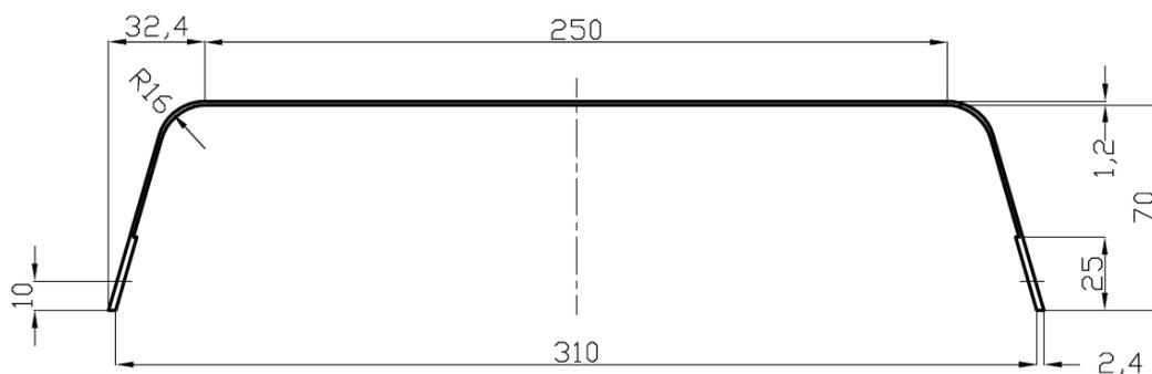
*Fig. 2. The scheme of a protective panel with the casing of trapezoid form with the height of 70 mm*
