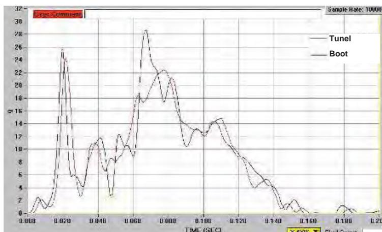
Fig. 12. Diagrams of deceleration constituents' courses „in the impact direction” (of chosen points) – Suzuki Swift
