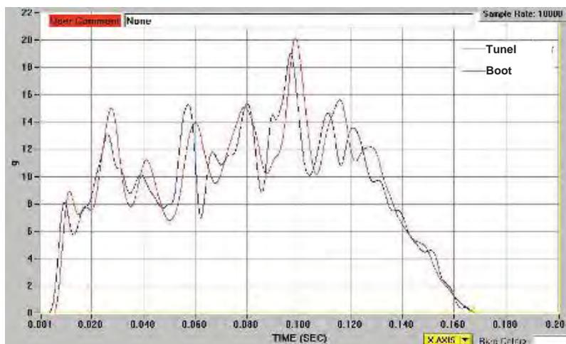
Fig. 6. Diagrams of deceleration constituents' courses „in the impact direction” (of chosen points) – Suzuki Swift
