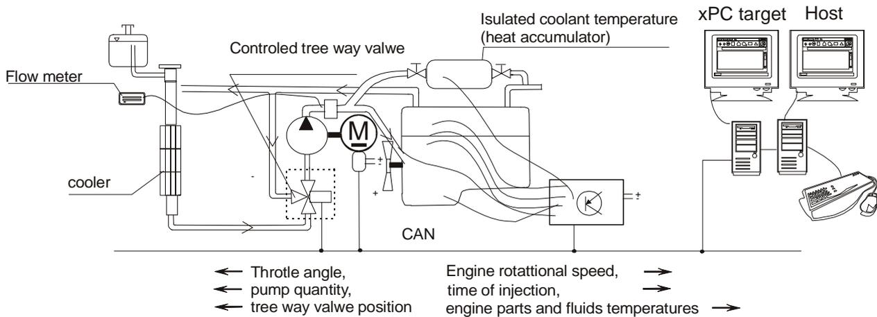
Fig. 5. Schematics of the developed test stand
