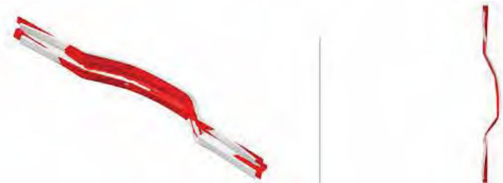
Fig. 9. Comparison of the road barrier's belt deformation (marked in red colour – experiment, light-gray colour – FEM)
