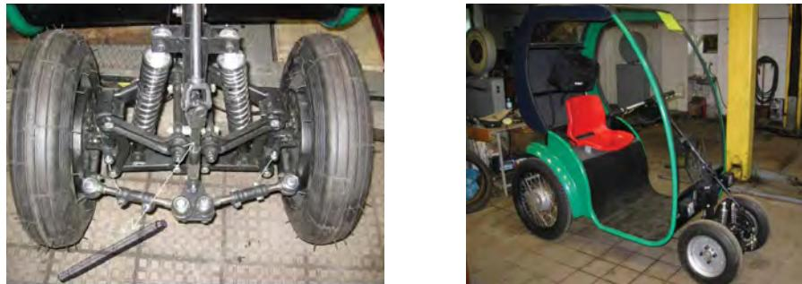
Fig. 6. Suspension with swivel axle [4]
