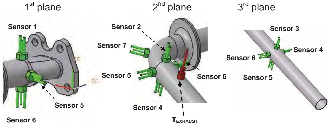
Fig. 10. Sensor positions in first, second and third measuring plane in the research exhaust pipe
