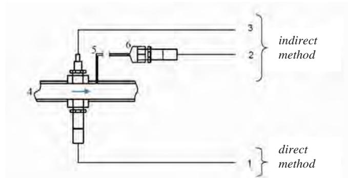
Fig. 6. Pressure measurement methods: 1 – piezoresistive sensor (channel 1; reference) – p1, 2 – piezoresistive sensor (channel 2; static part; tube connection) – p2, 3 – piezoelectric sensor (channel 3; dynamic part) – p3, 4 – intake manifold, 5 – tube ( $l=2000\text{mm}$ ), 6 – adapter
