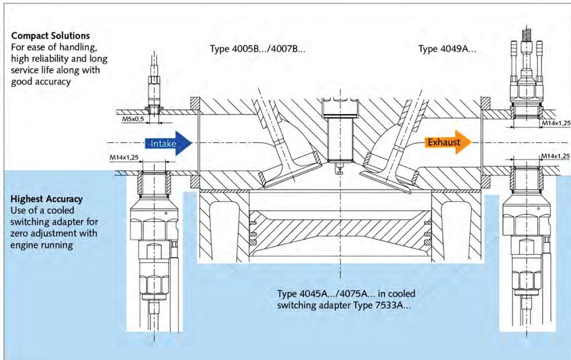
Fig. 4. State-of-the-art solutions of Kistler for low pressure measurement [10]
