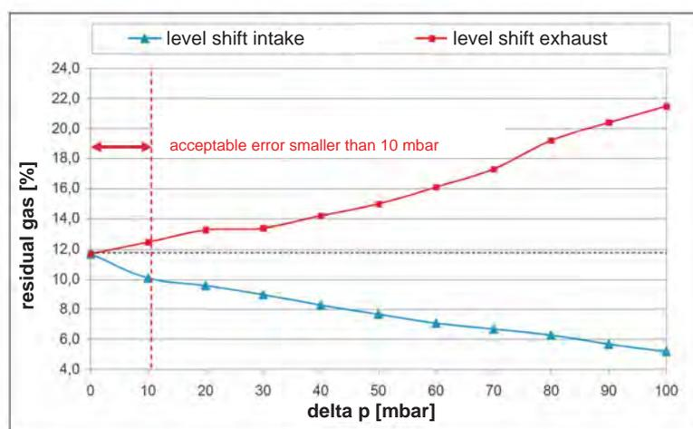
Fig. 1. Influence of the shift of pressure level in the inlet and outlet on the calculated residual gas content at 3000 rpm / part load [4]
