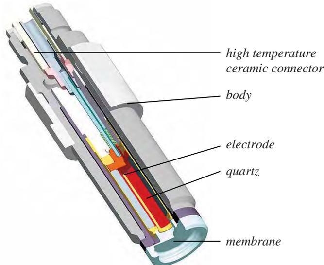
*Fig. 2. Principle of the piezoelectric sensor [5]*
