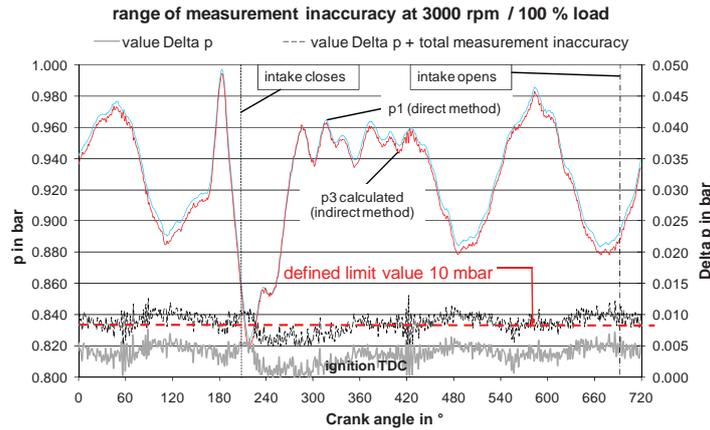
Fig. 7. Pressure curves with different measuring methods and resulting pressure differences
