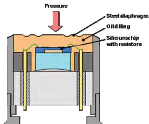
*Fig. 3. Principle of the piezoresistive sensor [4]*
