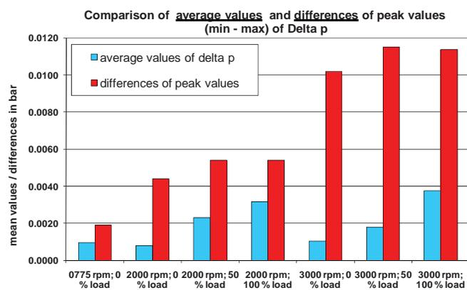
Fig. 8. Comparison of mean values and peak value differences of delta p
