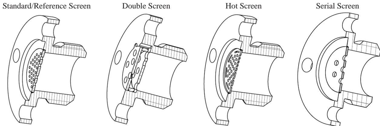
Fig. 14. Different types of screens which have been studied for best sensor performance
