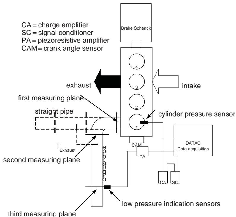
Fig. 9. Measuring set up for investigation of the exhaust blow off on Mercedes M111
