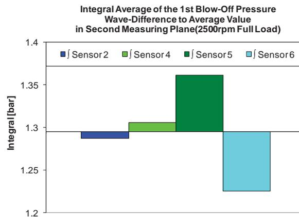
Fig. 12. Overview of pressure situation in second measuring plane (approx. 60°C blow off window averaged)
