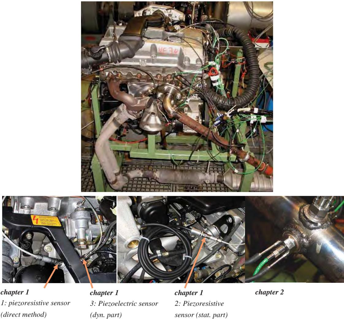
Fig. 5. Mercedes engine on the test stand and zoom on a measuring plane (chapter 2) and the intake arrangement (chapter 1)
