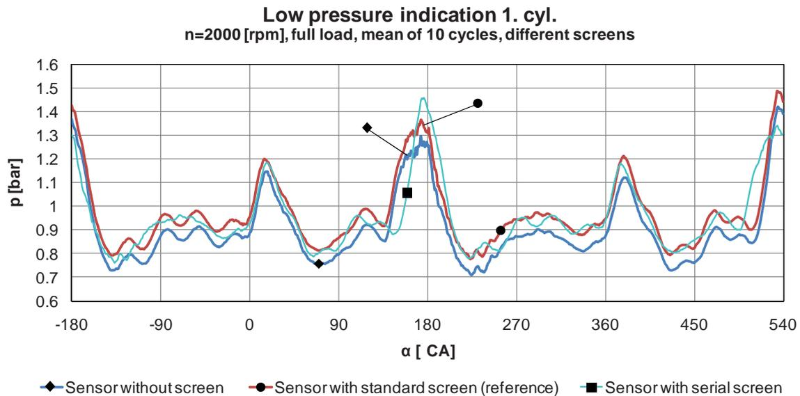
Fig. 15. Pressure curves with different screens, 2000 rpm / full load
