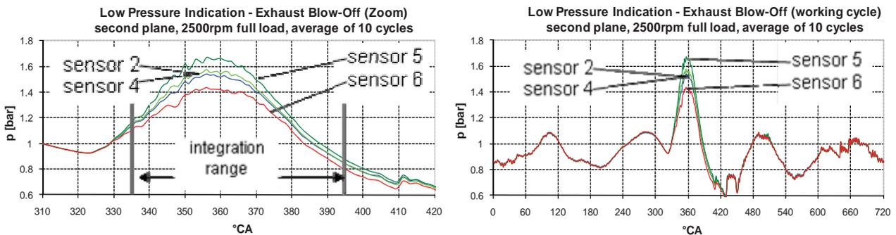
Fig. 11: Exhaust blow off in working cycle and zoom showing sensor differences (second plane)
