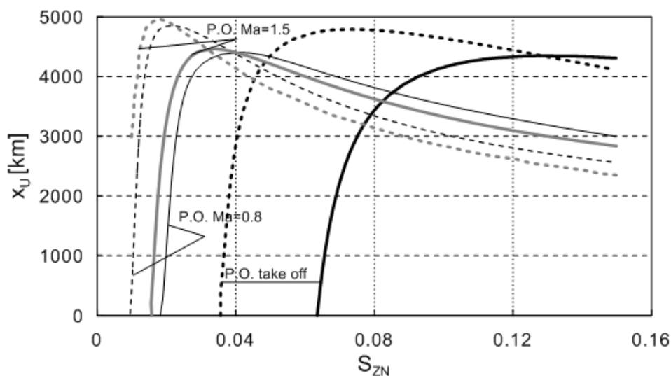
Fig. 3. Influence of choice of engine calculation point and  $S_{ZN}$  on the conventional range of aircraft performed for  $Ma=1.5$   $H=5000$  (full line) and  $Ma=1.5$   $H=18000$  (broken line)
