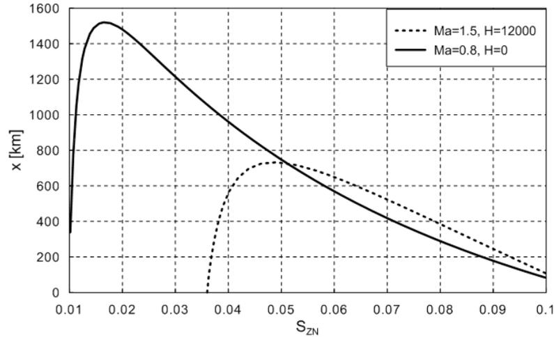
Fig. 1. Influence of the parameter of engine adjustment to the aircraft  $S_{ZN}$  on the theoretical range for the subsonic flight (full line) and supersonic flight (broken line)
