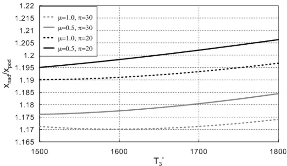
Fig. 7. Influence of temperature  $T_3$  and  $\mu$  as well as  $\pi$  for the relative range  $x_{pod}/x_{nad}$ . Subsonic flight  $Ma=0.8$ , supersonic flight  $Ma=1.6$ ,  $H=12000$  m
