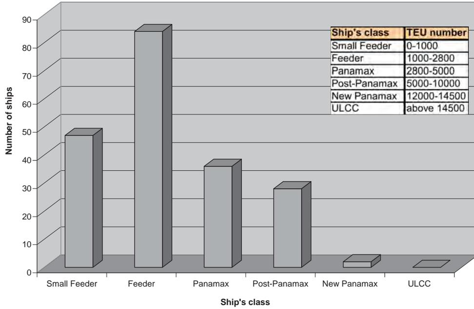
Fig. 2. Database structure with container carriers' classification
