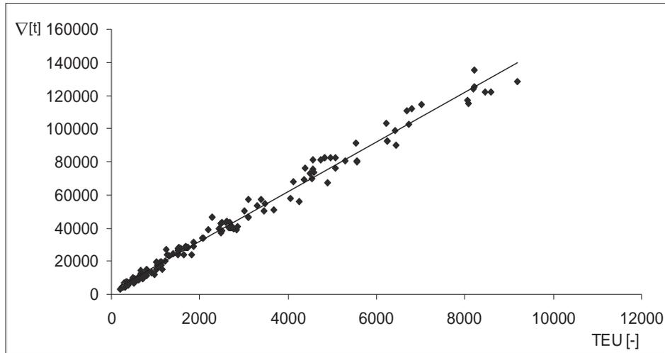
Fig. 4. Linear relation between container vessels displacement and container number (TEU)
