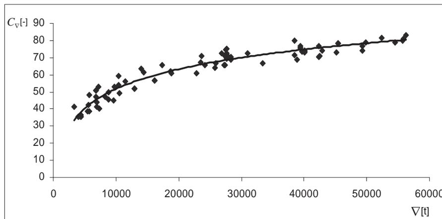
Fig. 3. Determination of proportionality factor (C) for ship's displacement in first range
