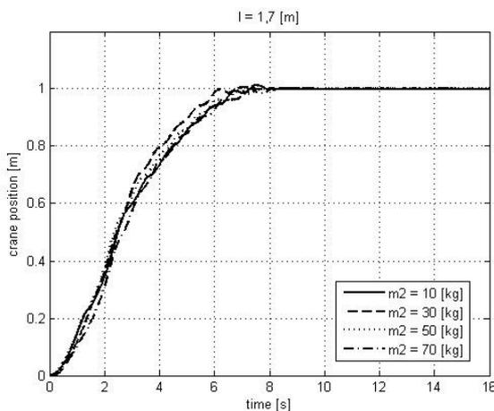
Fig. 7. The crane position for  $l = 1.7$  [m] and  $m_2 = \{10, 30, 50, 70\}$  [kg]
