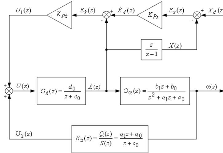
Fig. 3. The time-discrete crane position and speed, as well as the load swing control system
