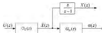
Fig. 1. The assumed parametric model of a crane dynamic consisting of two models expressed in a form of discrete transfer functions  $G_{\dot{x}}(z)$  and  $G_{\alpha}(z)$
