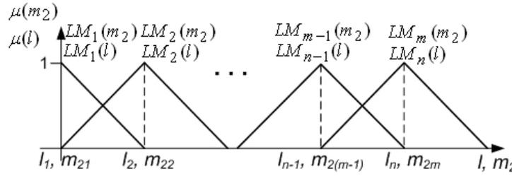
Fig. 2. The triangular membership functions defined for  $l$  and  $m_2$  input variables of TSK fuzzy estimator
