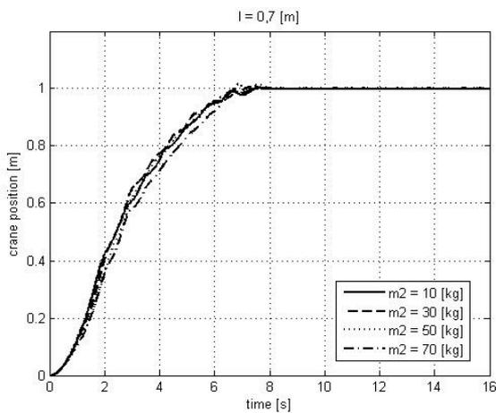
Fig. 5. The crane position for  $l = 0.7$  [m] and  $m_2 = \{10, 30, 50, 70\}$  [kg]
