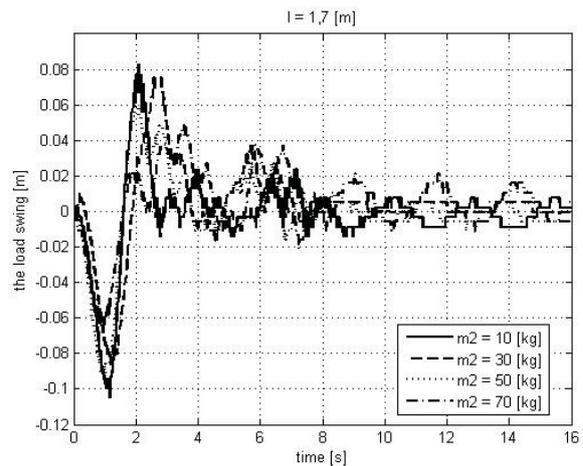
Fig. 8. The load swing for  $l = 1.7$  [m] and  $m_2 = \{10, 30, 50, 70\}$  [kg]
