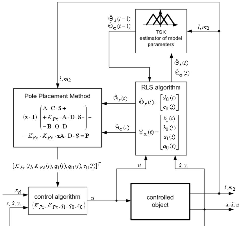
Fig. 4. The indirect adaptive pole placement crane control system with the TSK fuzzy estimator of crane model parameters
