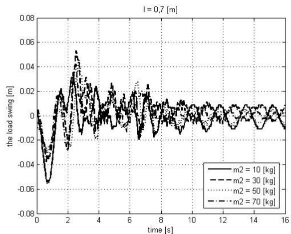
Fig. 6. The load swing for  $l = 0.7$  [m] and  $m_2 = \{10, 30, 50, 70\}$  [kg]
