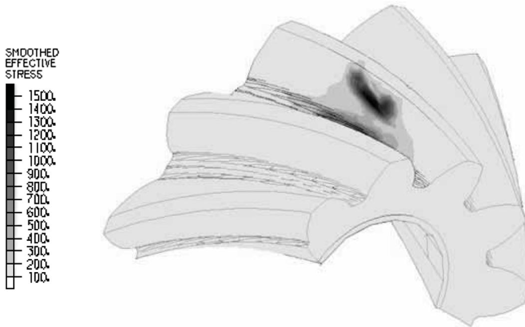
Fig. 3. The distribution of reduced stresses in a selected analytical step for the pinion
