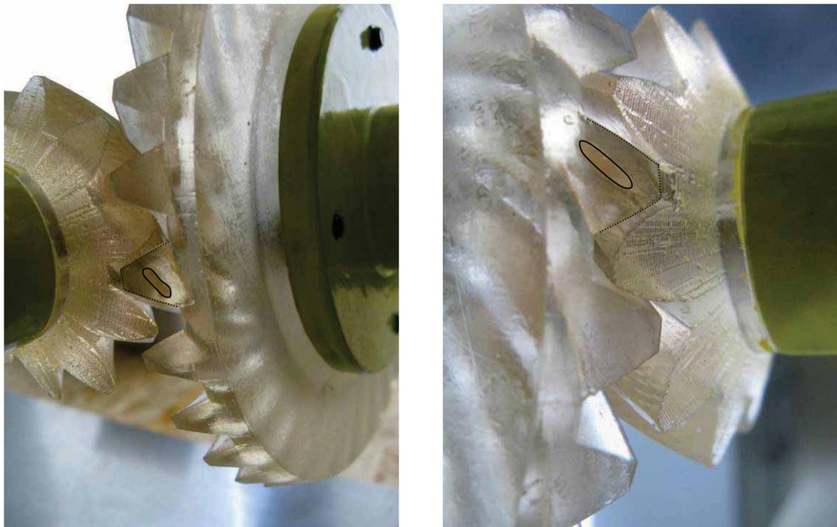
*Fig. 8. An instantaneous contact track of bevel gear wheels marked on the test stand*
