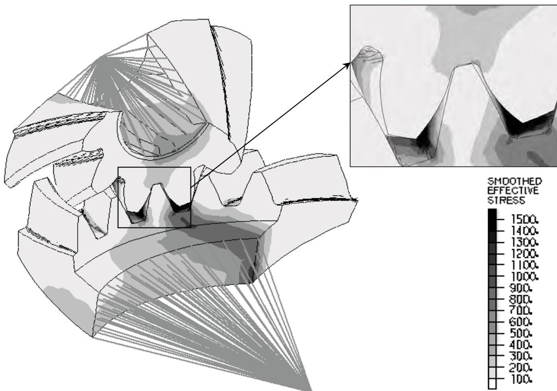
Fig. 2. The reduced stresses (according to Misses) in overall sight and on a detail of wheel model and pinion model
