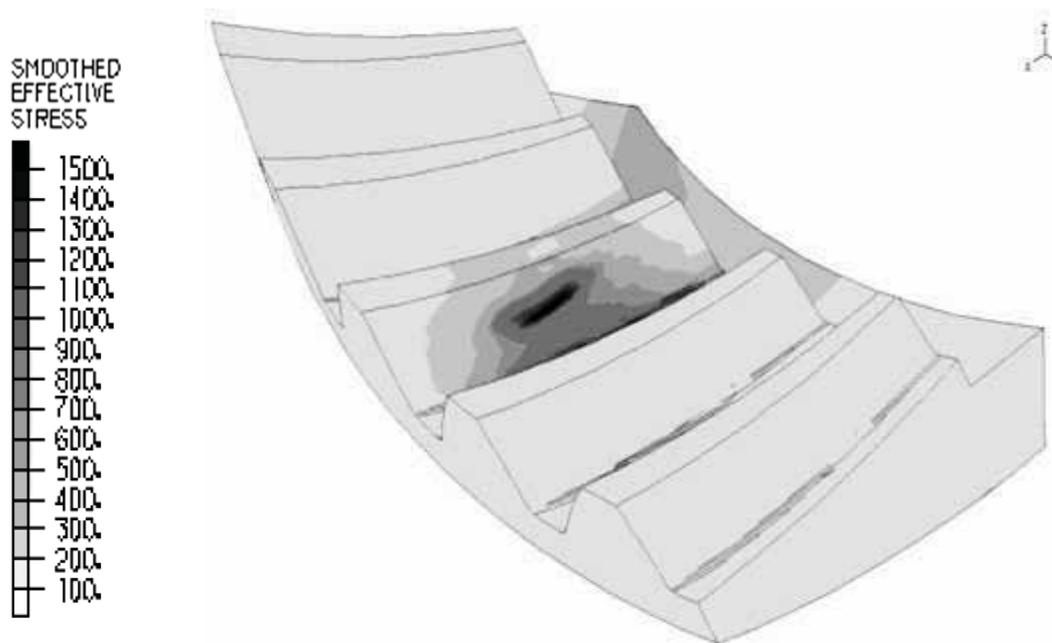
Fig. 4. The distribution of reduced stresses in a selected analytical step for the wheel
