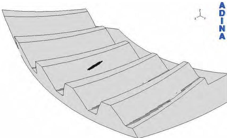
Fig. 6. Instantaneous contact track on the side surface of the wheel's tooth
