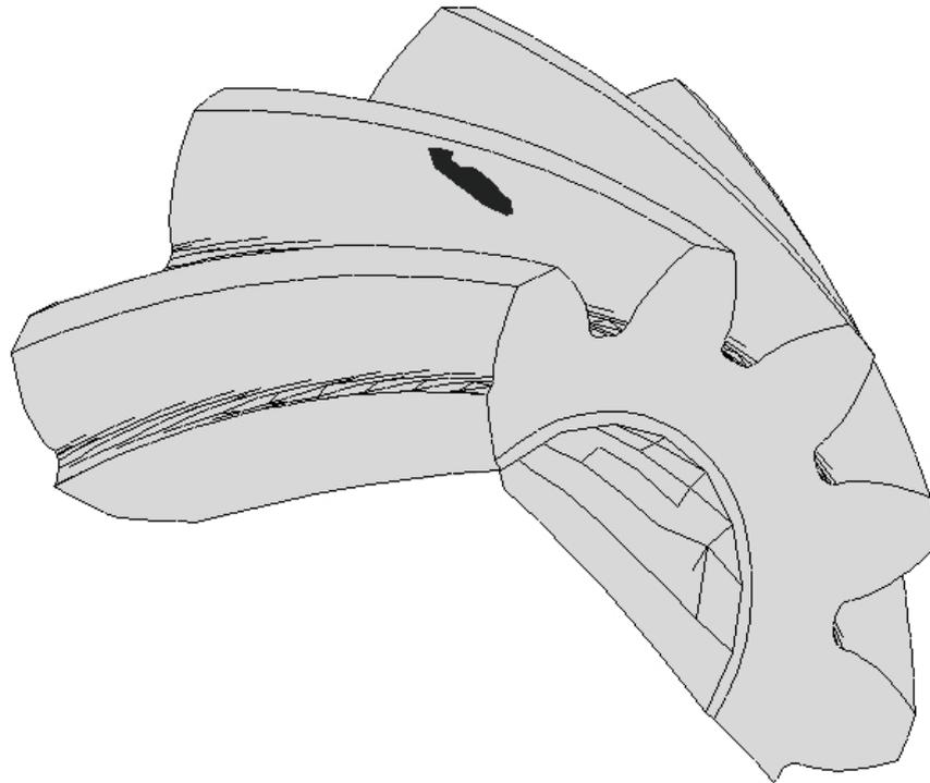
Fig. 5. Instantaneous contact track on the side surface of the pinion's tooth
