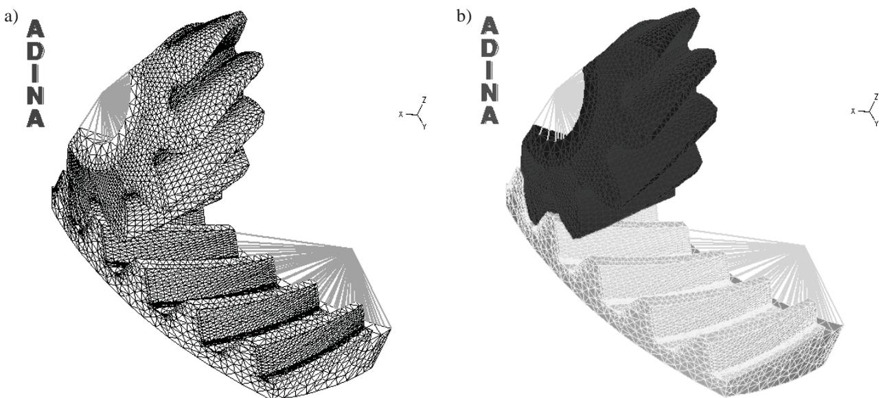
Fig. 1. The Wheel models under the digitizing process: a) with visible division into finite elements, b) with elements differentiated by two shades of grey
