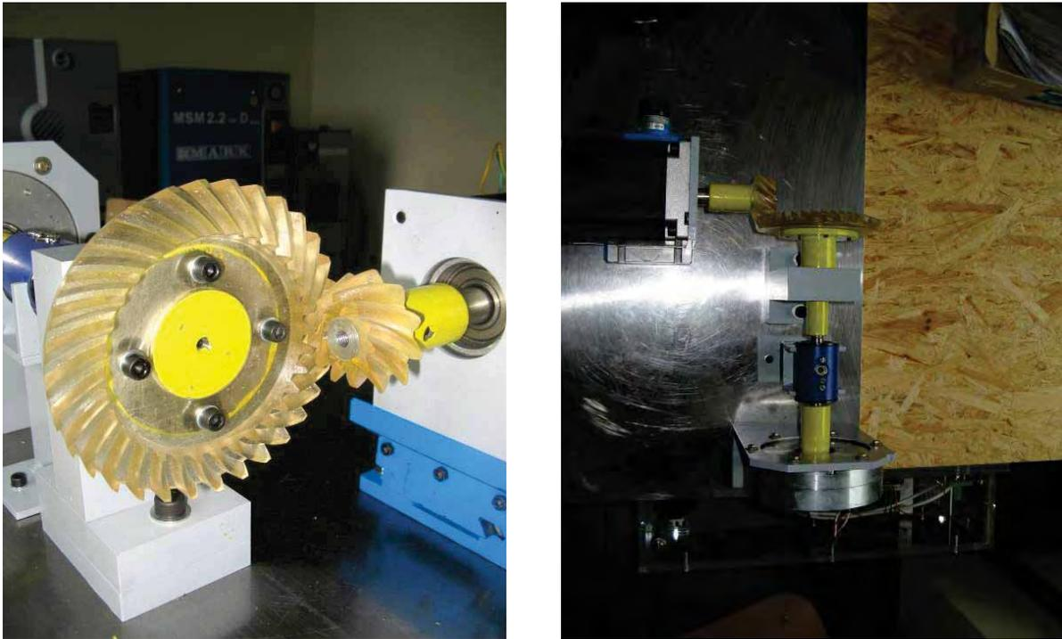
*Fig. 7. A test stand for examining the contact track of bevel gear wheels*
