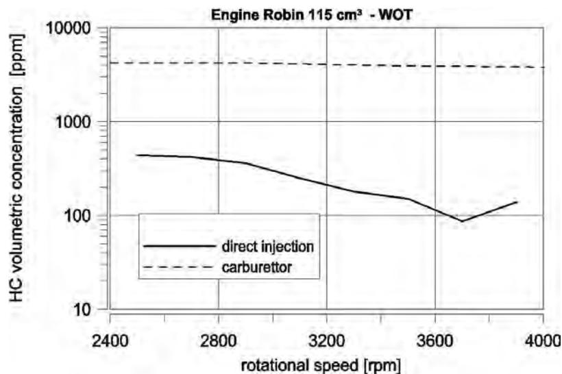
Fig. 5. Comparison of hydrocarbon volumetric concentration in exhaust gases in two-stroke engine for carburetted version and direct fuel injection version
