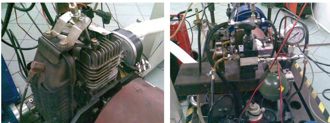
Fig. 2. Photos of experimental stand with direct fuel injection two-stroke engine
