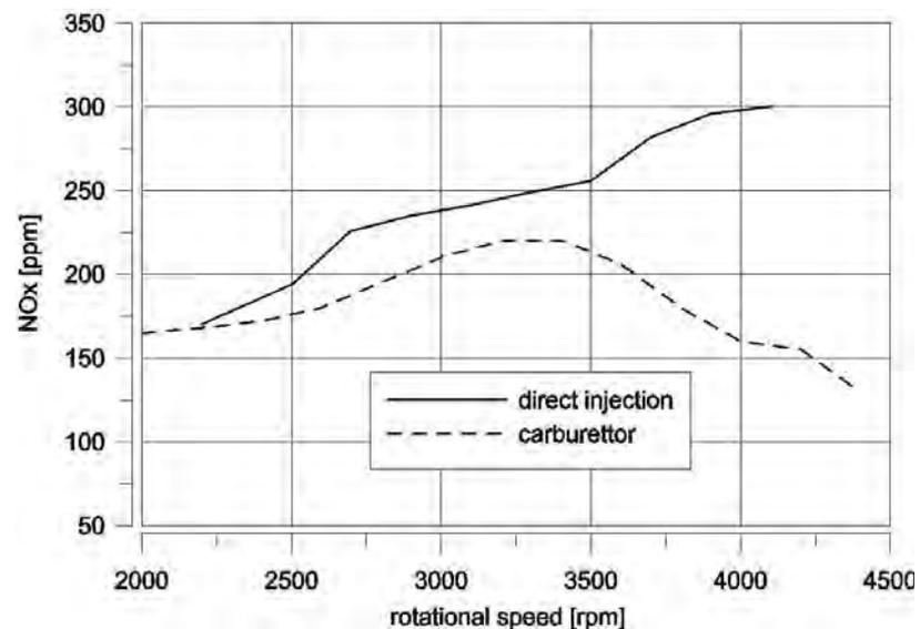
Fig. 7. Comparison of NOx volumetric concentration in exhaust gases in two-stroke engine for carburetted version and direct fuel injection version
