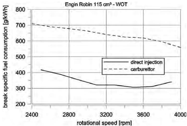
Fig. 4. Comparison of break specific fuel consumption of engine in carburetted version and direct fuel injection version
