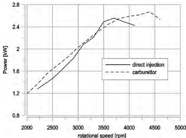
Fig. 3 Comparison of engine power in carburetted version and direct fuel injection version
