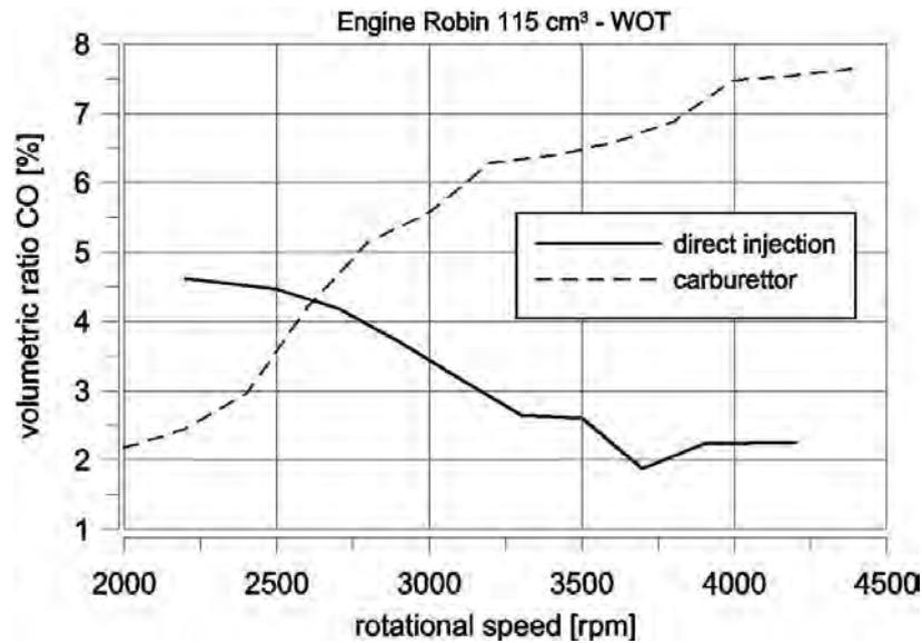
Fig. 6. Comparison of carbon monoxide volumetric concentration in exhaust gases in two-stroke engine for carburetted version and direct fuel injection version
