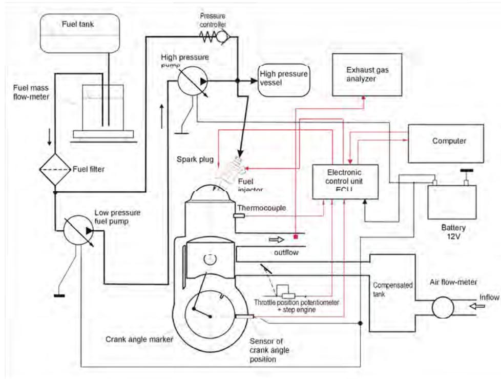
Fig. 1. Diagram of direct fuel injection two-stroke engine on experimental stand
