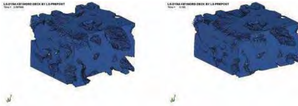
Fig. 8. Deformations of the sample in numerical compression test
