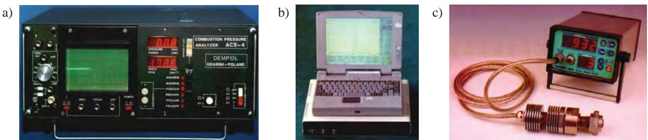
Fig. 1. Portable pressure analyzers developed and applied in Poland: a) – ACS-4 analyzer, b) – MA2000 analyzer, c) – UNITEST 203 analyzer
