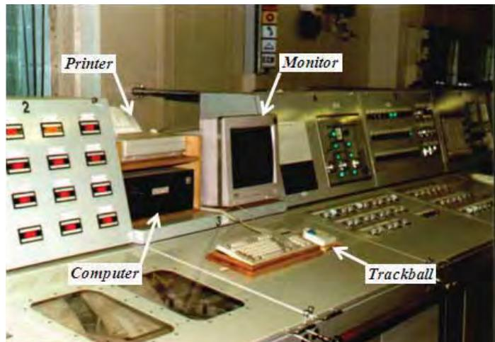
Fig. 3. Hardware of monitoring-diagnostic system on an operator desktop on bulk carrier
