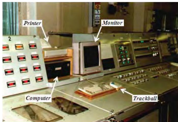
Fig. 3. Hardware of monitoring-diagnostic system on an operator desktop on bulk carrier
