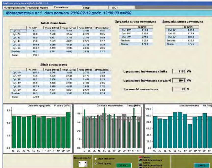
Fig. 6. Presentation of tables and bar charts of parameters on the monitor screen of GMVH motor compressor monitoring-diagnostic system
