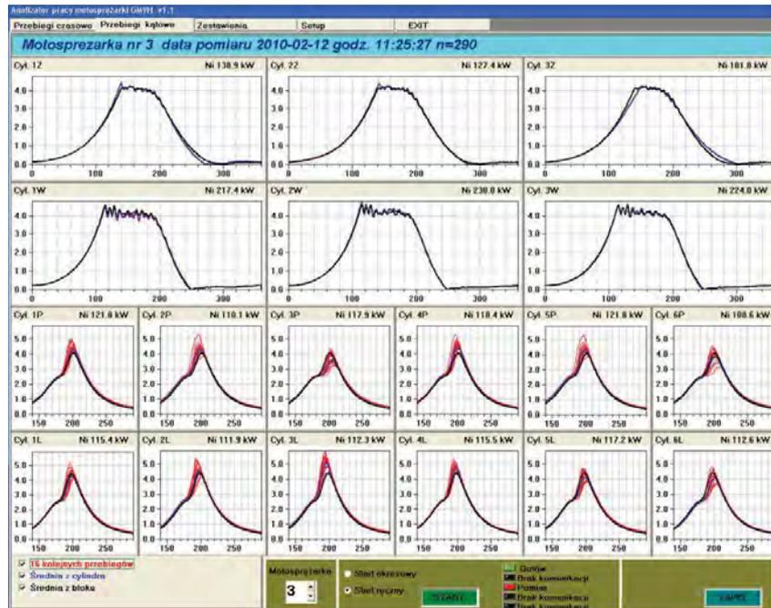
Fig. 5. Main menu of pressure analyzer of GMVH motor compressor monitoring-diagnostic system, presented in on-line mode
