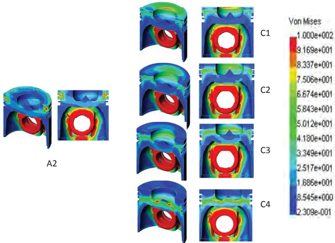
Fig. 6. Stresses distribution in standard piston A2 and different version of composite piston C1, C2, C3, C4
