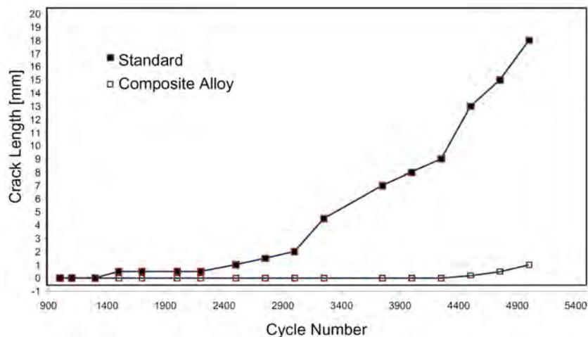
Fig. 7. The resistance of investigated materials on thermal shocks
