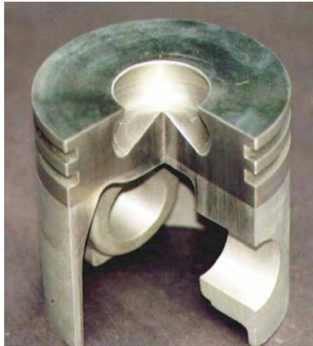
Fig. 3. Composite piston locally reinforced
