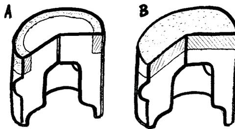
Fig. 2. Schemas of a installed local piston reinforcements with composite ceramic inserts of two types
