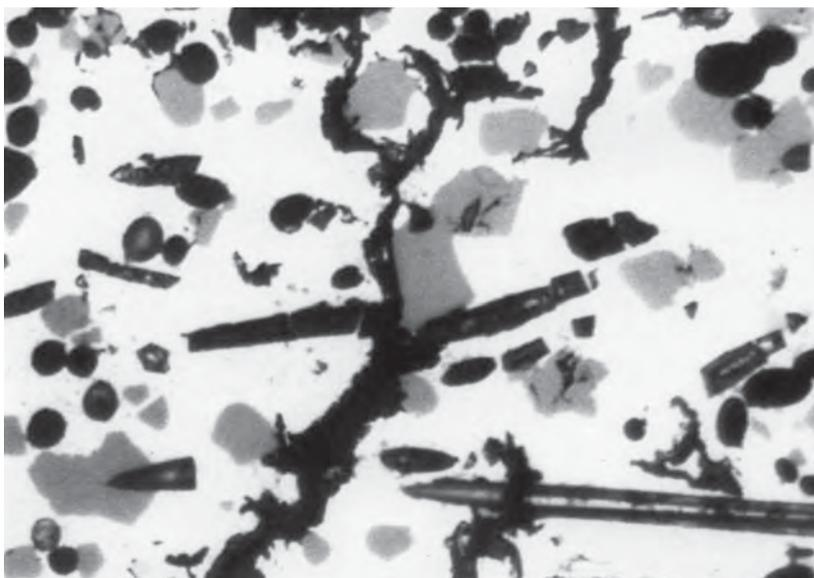
*Fig. 9. The microstructure of composite alloy after investigations of the material resistance on thermal shocks. Magn.500x*
