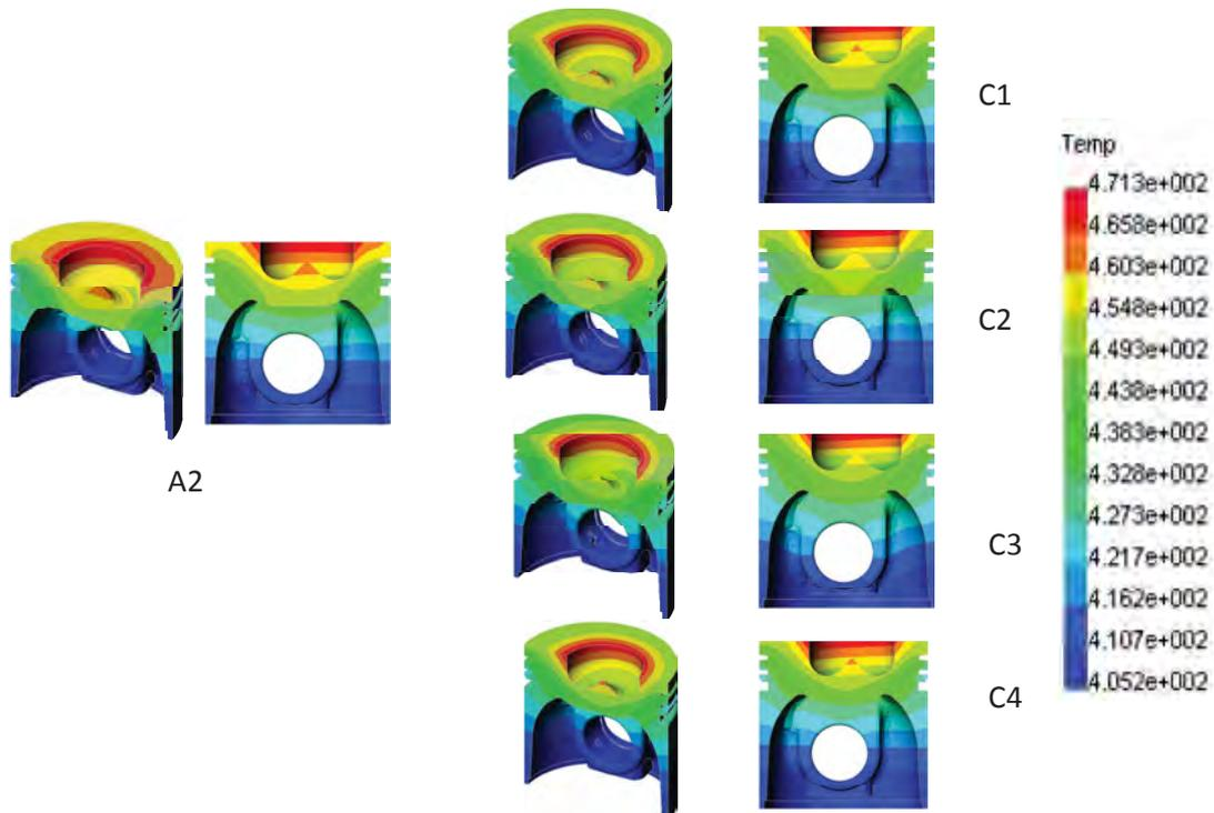
Fig. 5. Temperature distribution in standard piston A2 and different versions of composite pistons C1, C2, C3, C4
