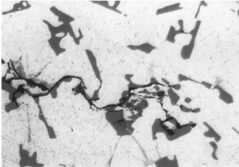
*Fig. 8. The microstructure of standard alloy AK 12 after investigations of the material resistance on thermal shocks. Magn. 500x*
