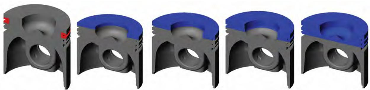
Fig.4. Five versions of engine pistons, on the left: standard piston (A2), the next: composite pistons (C1, C2, C3, C4)
