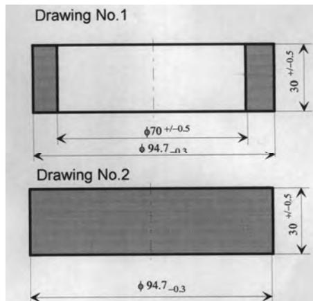
Fig. 1. Drawings of the inserts for local pistons reinforcements
