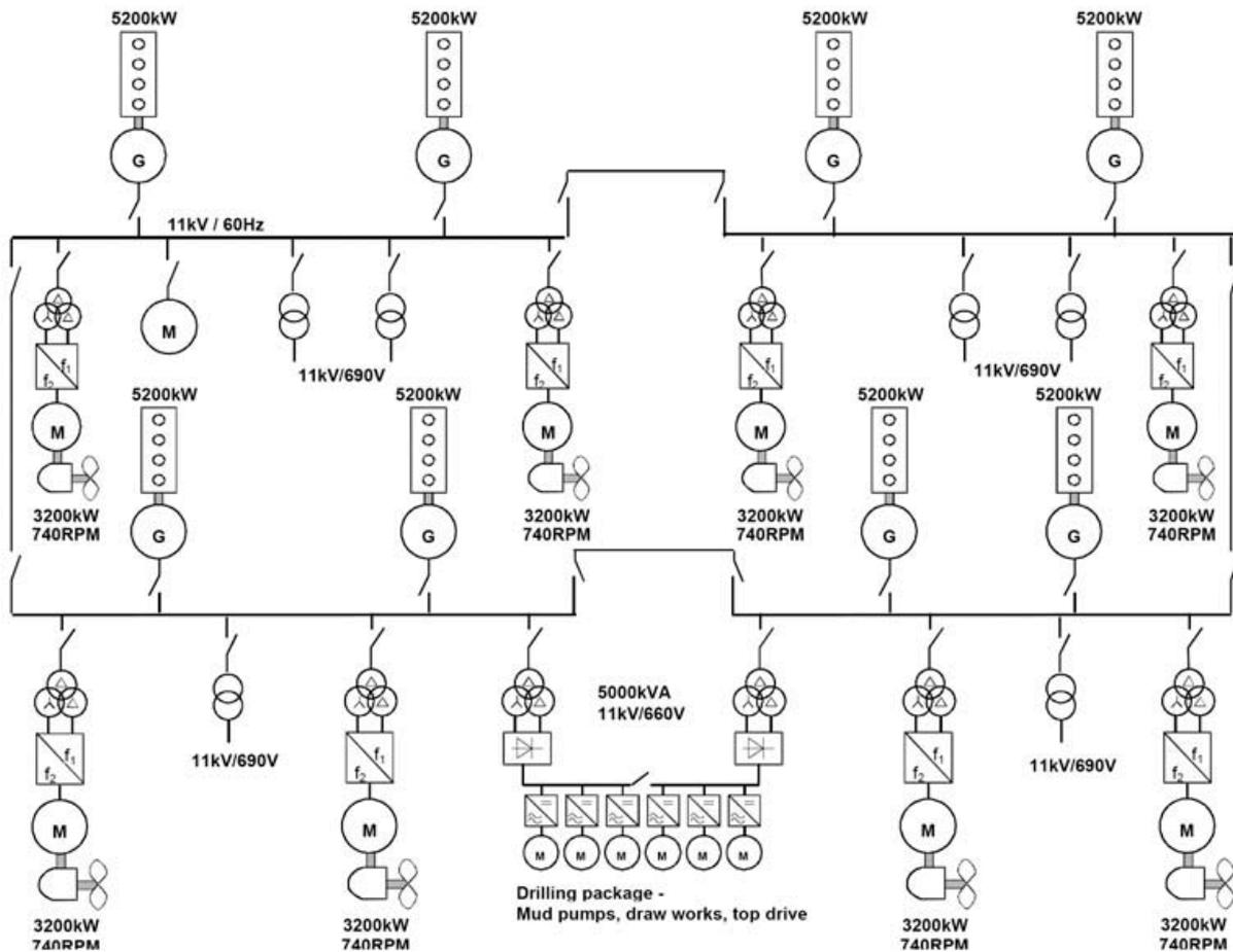
Fig. 5. Power system configuration for drilling vessel [1]. Single line diagram for a DP Class 3 drill rig with a four-split power system - ring network
