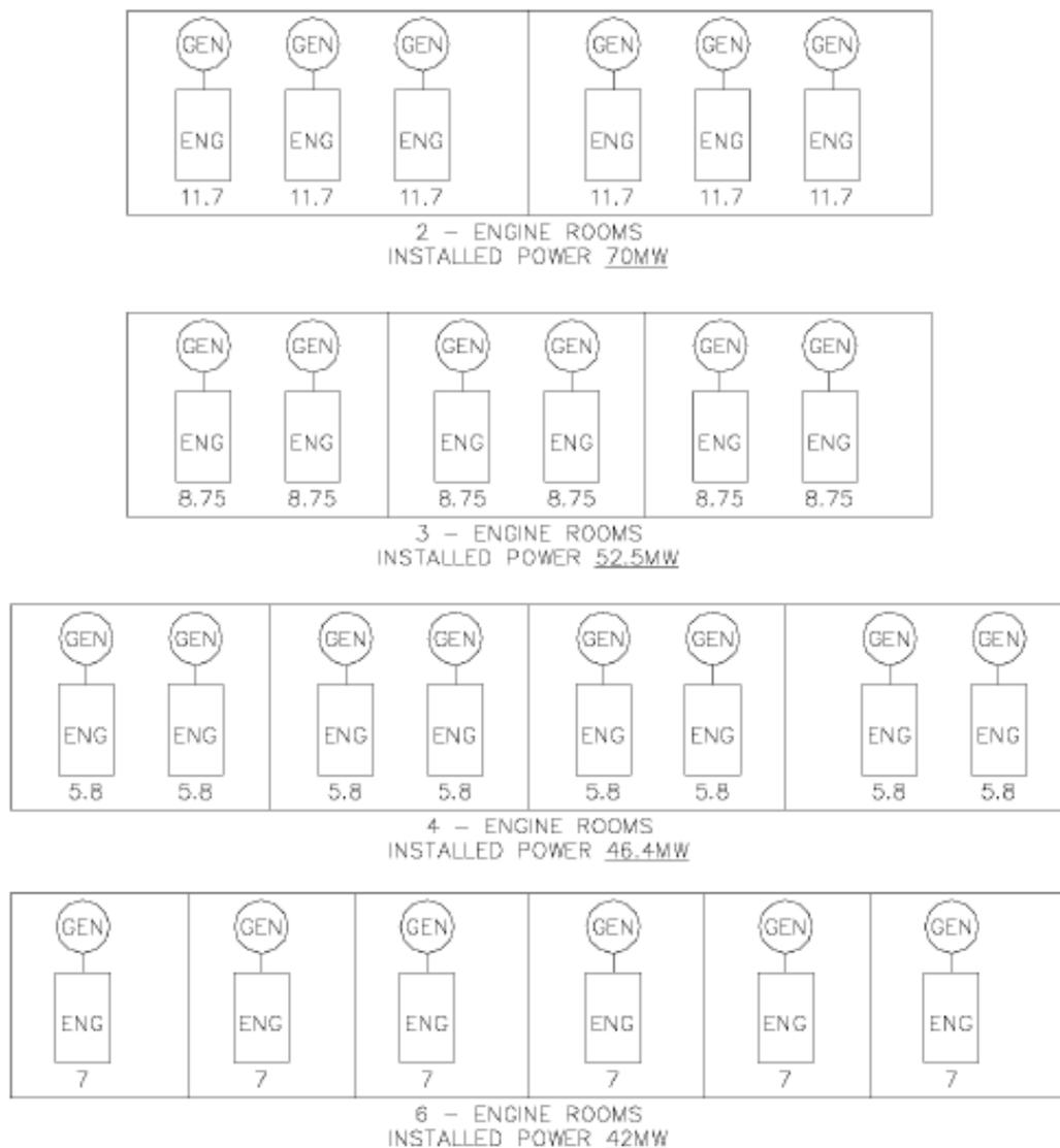
Fig. 6. Power system configuration for drilling vessel [3]
