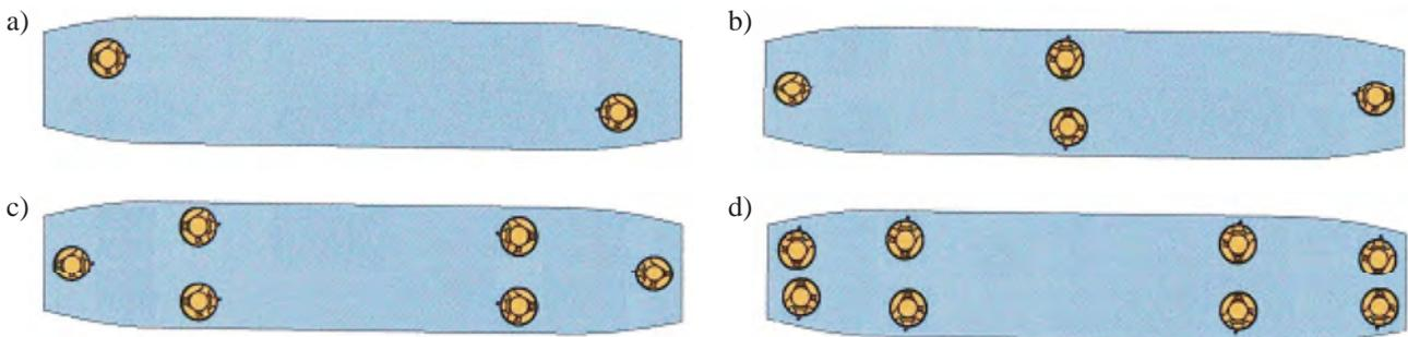
Fig. 2. Propositions of multi-element propulsion arrangement for DP systems: a) the minimum, b) for discussion, c) for analysis, d) for two engine rooms
