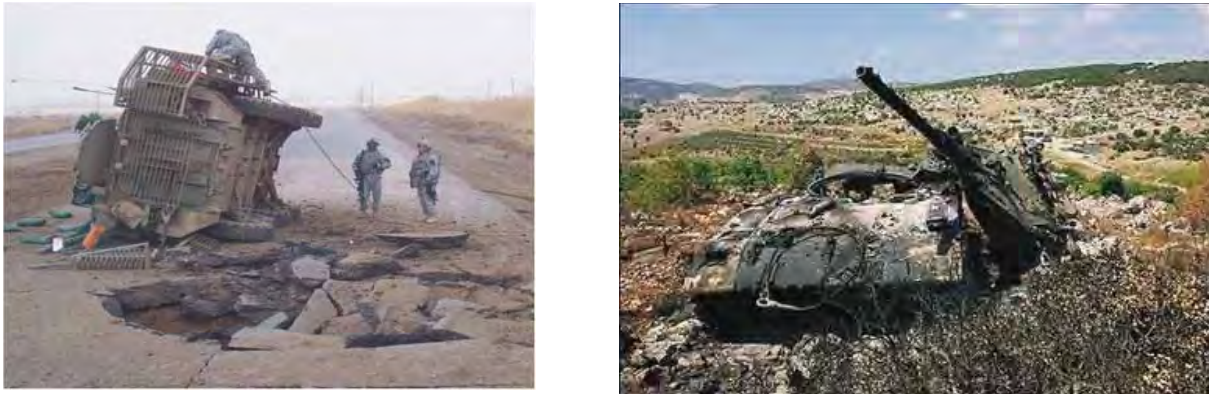
Fig. 3. Effect of the impact of IED on vehicles of different classes [5]
