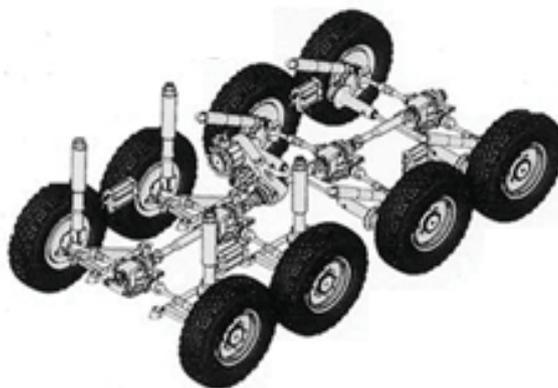
*Fig. 2. Drive system scheme*
