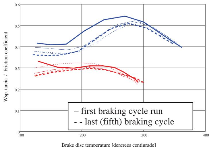
Fig. 13. Friction characteristics of the composite brake disc (20 % SiC - red line) and cast iron (blue line) with truck brake shoe lining (JU-1) and brake line pressure of 9 bars
