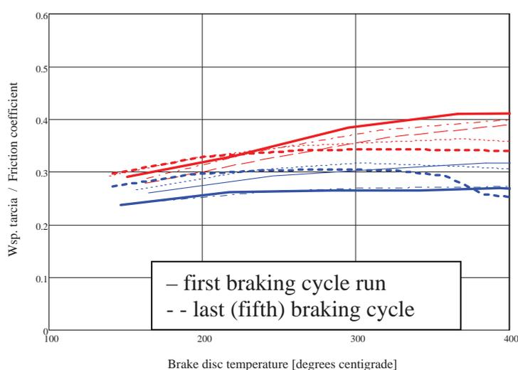
Fig. 14. Friction characteristics of the composite brake disc (20 % SiC - red line) and composite brake disc with fly ash (blue line) with brake pads for composite brake disc (LE)
