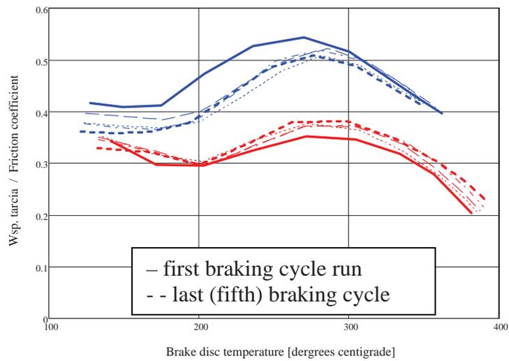
Fig. 11. Friction characteristics of the cast iron brake disc with truck brake shoe lining (JU-1) and different brake line pressures (15 bar - red line; 9 bar - blue line)
