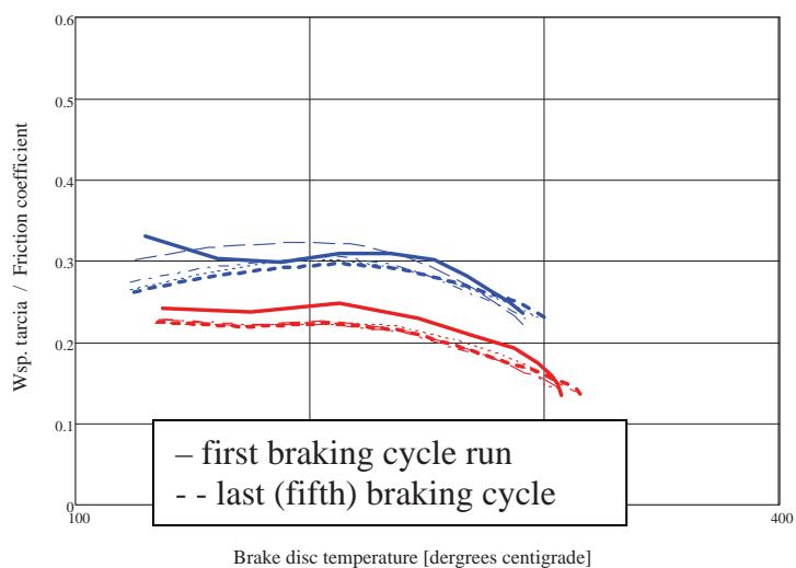
Fig. 9. Friction characteristics of the composite brake disc (20 % SiC) with truck brake shoe lining (JU-1) and different brake line pressures (15 bar - red line; 9 bar - blue line)
