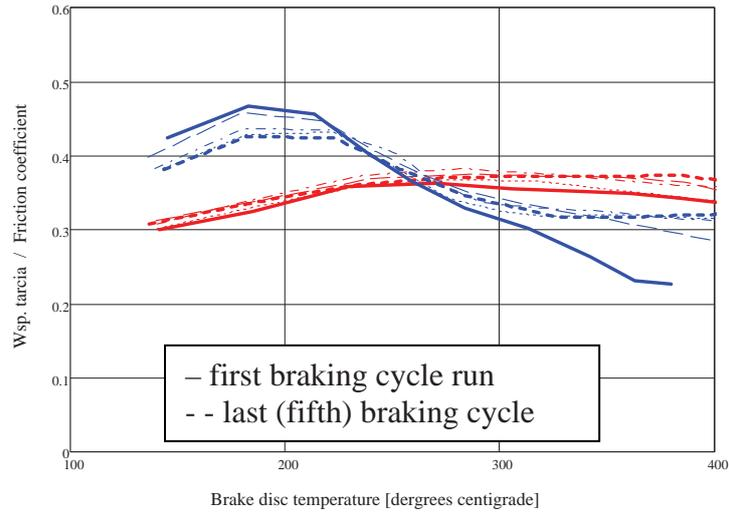
Fig. 7. Friction characteristics of the composite brake disc (20 % SiC - red line) and cast iron brake disc (blue line) with “racing” brake pads (EBC-2)
