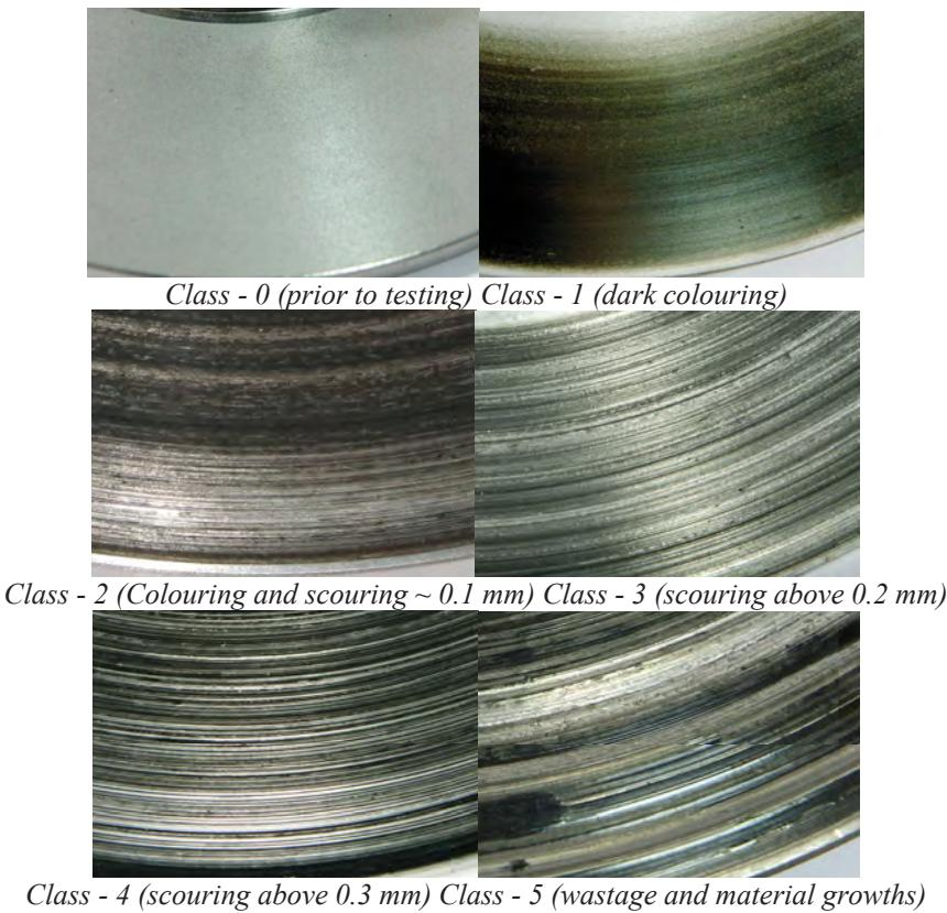
*Fig. 6. Wear classes of the brake disc surface*
