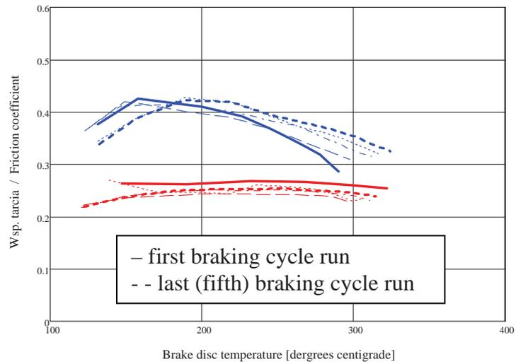
Fig. 8. Friction characteristics of the composite brake disc (20 % SiC - red line) and cast iron brake disc (blue line) with truck brake pads (BR)
