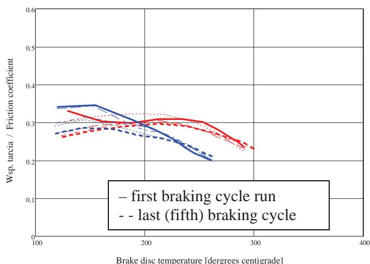
Fig. 12. Friction characteristics of the composite brake disc (20 % SiC - red line; 30 % SiC - blue line) with truck brake shoe lining (JU-1) and brake line pressure of 9 bar
