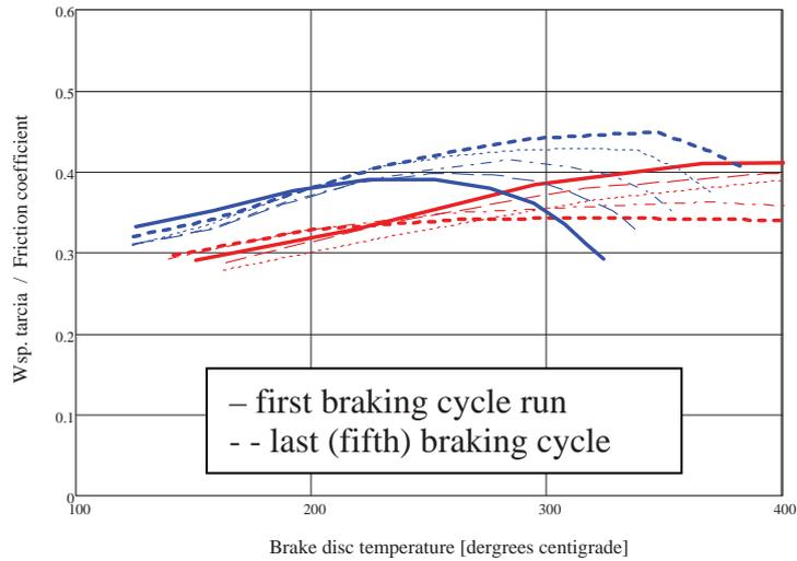
Fig. 10. Friction characteristics of the composite brake disc (20 % SiC) with brake pads for composite brake disc (LE) and different brake line pressures (15 bar - red line; 9 bar - blue line)
