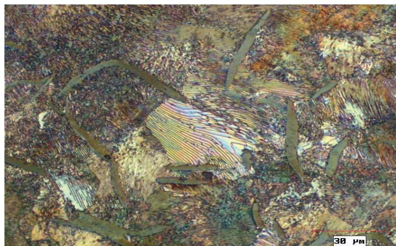
Fig. 1. Structure of cast iron (500 x magnification)
